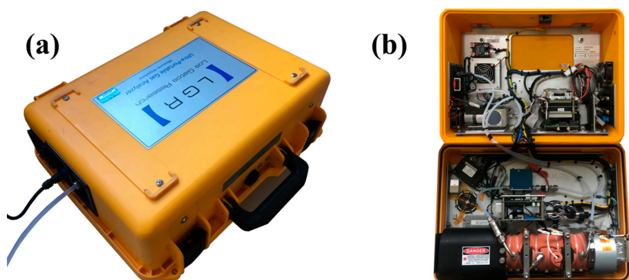
Figure A2. (a) The Ultra-portable Greenhouse Gas Analyzer (UGGA) with its lid closed and an air inlet attached; (b) the UGGA with its lid open.
