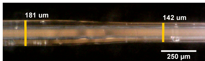
Fig. 5: Etched Zeonex POF (annealed). The fiber has been immersed in trichloroethylene for 6 minutes. The fiber diameter was etched from 181 \mu\text{m} to 142 \mu\text{m} .
