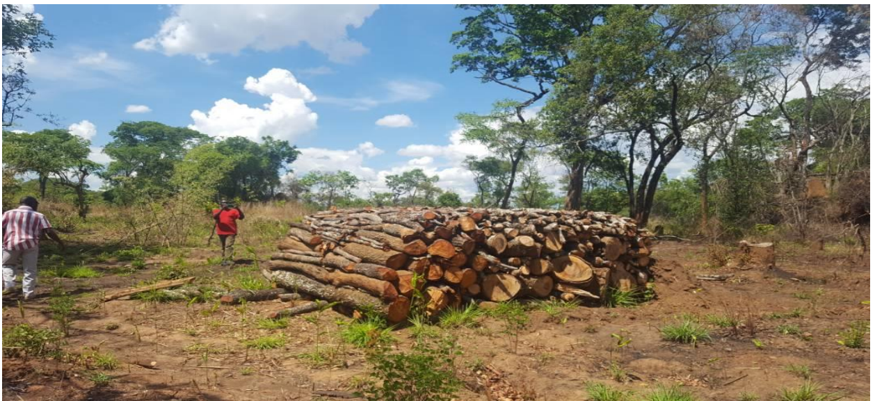
Figure 5.16 (b): Tree logs before they are covered with earth to make a kiln
