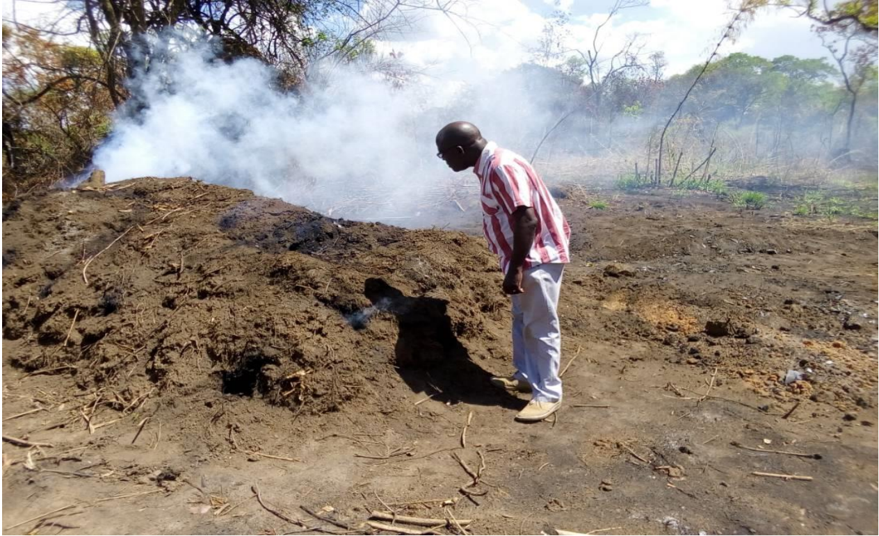
Figure 5.15: Charcoal being produced in earth mound kiln
