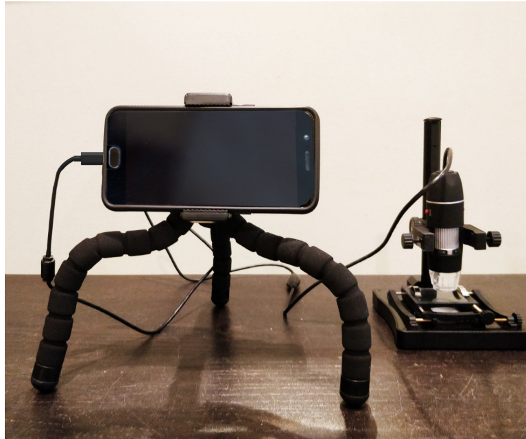
Fig 1. An Android smartphone mounted on a tripod connected to the UVC used in this study, which is mounted in a microscope stand with X-Y stage.
