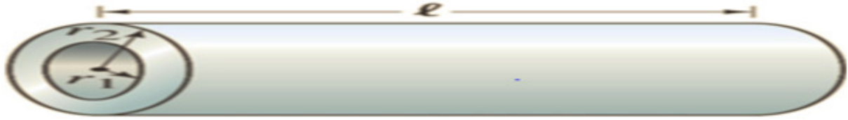
Figure 5: A hollow cylinder with length L , the internal and external radius of r_1 and r_2 respectively.
