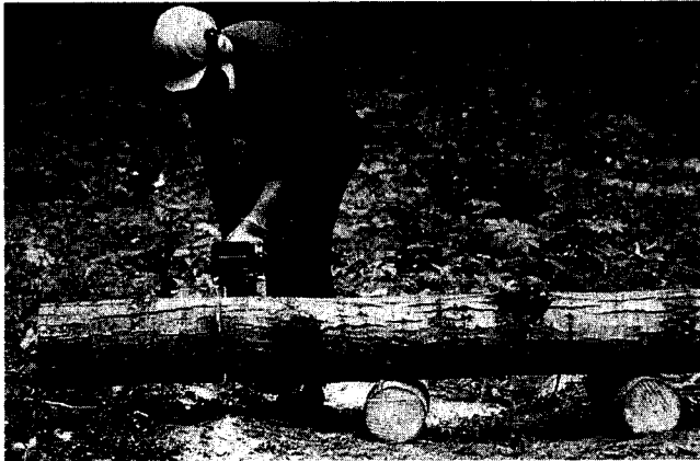
Figure 7. Identifying the location of tension and compression wood in a trunk will make it easier to buck without binding the saw bar.
