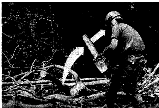
Figure 2. A kickback can occur in less than one-tenth of a second, faster than the human brain can respond.
