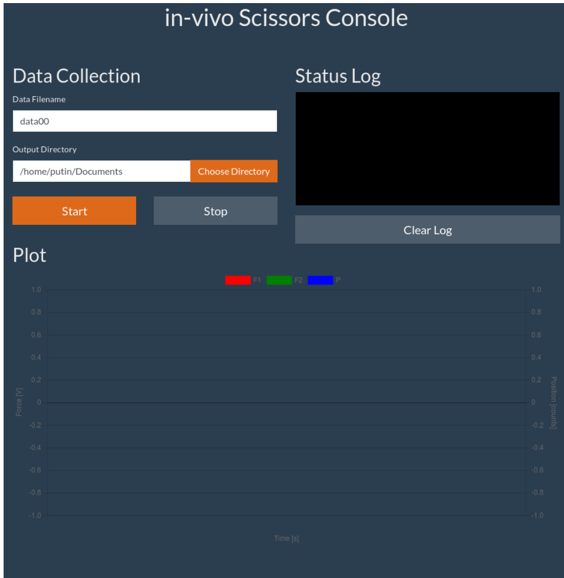
Figure 2.12: Screenshot of data collection GUI dubbed the “Scissors Console”. Users can set the data filename and folder path. Buttons control when to start and stop data collection, as well as log clearing. A plot on the bottom of the screen displays the incoming data in real-time, allowing users to immediately be aware of data collection issues during the experiment.
