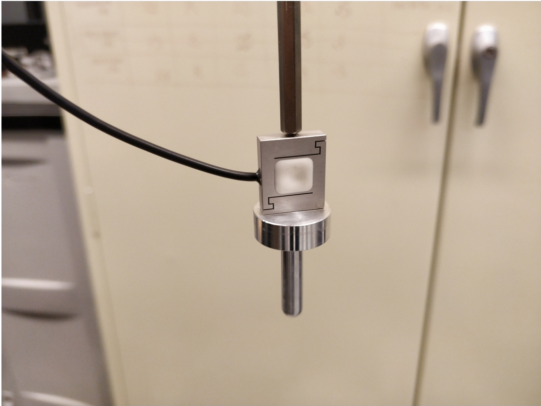
Figure 2.6: Close up photo of the spherical indenter tip and load cell (Futek LSB210 submersible load cell).
