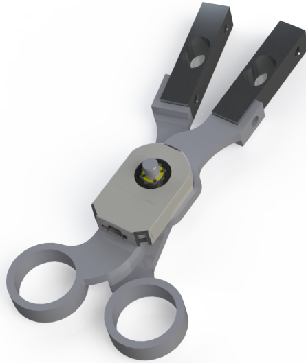
Figure 2.10: CAD render of In-vivo Mechanical Grasping Device instrumented with encoder and load cells.
