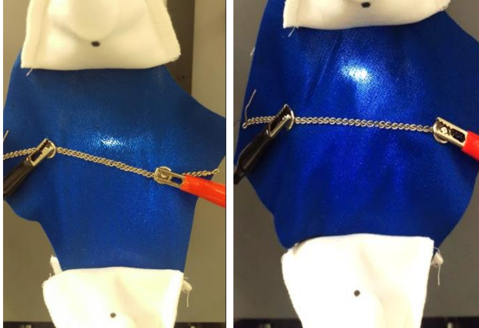
Figure 46. (Left) Test setup for 2-way 30° chainstitch with force applied at 60° (Right) 2-way 30° chainstitch with force applied at 90°
