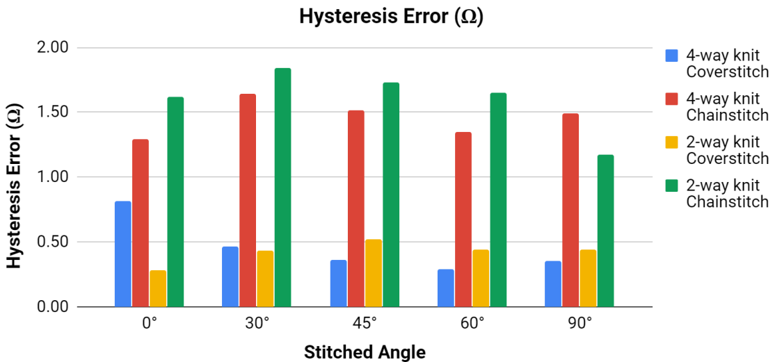
Figure 45. Comparing Hysteresis Error
