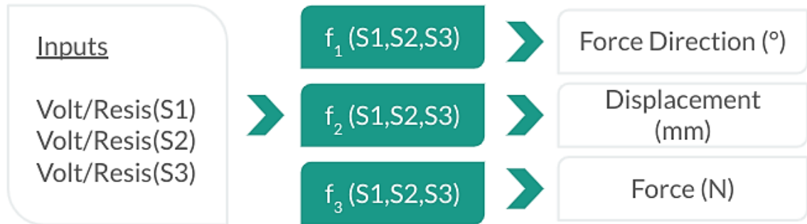
Figure 55. Schematic of using the measurements of the 2D Strain Rosette to predict Force Direction, Displacement, and Force
