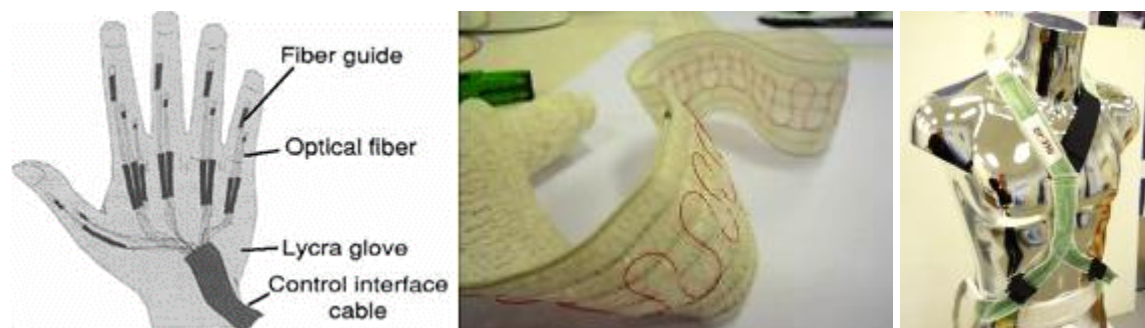
Figure 8. (Left) DataGlove by VPL (Zimmerman et al., 1986) (Center) POF sensor embedded into elastic stretch band (Narbonneau et al., 2010) (Right) Respiratory sensing harness for the MRI (Narbonneau et al., 2010)
