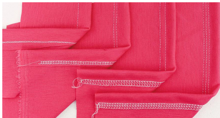
Figure 13. (Top left to bottom right) The chainstitch; narrow two thread bottom coverstitch; regular 2-thread bottom coverstitch; 3-thread bottom coverstitch
