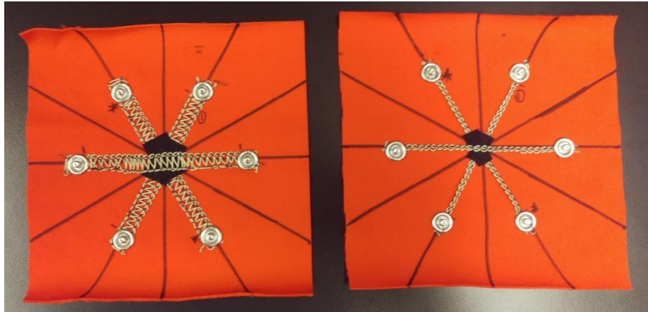
Figure 56. (Left) 4-way Coverstitch Rosette (Right) 4-way Chainstitch Rosette
