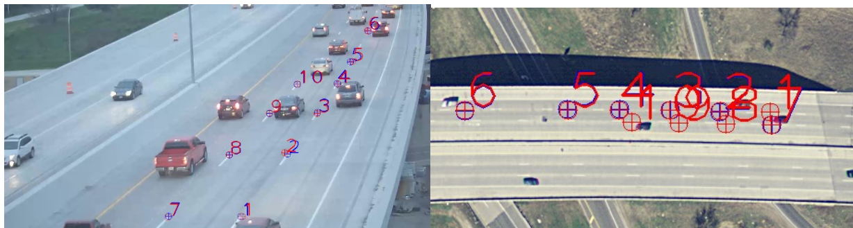
Figure 4.2 Example of points used to generate the homography for one of the TH-61 layouts. The left image is the camera frame, and the right image is the aerial image. On each image, the blue points are the original points selected on that image, while the red points are the corresponding points projected from the other image using the computed homography.
