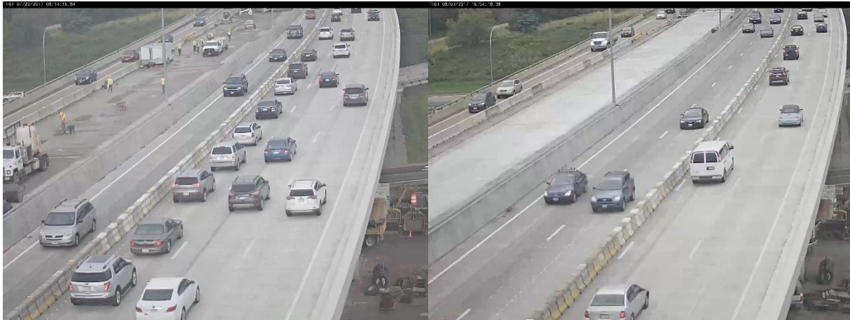
Figure 4.3 Example of two camera views/layouts that were considered similar enough to use the same configuration. In this case, the error from using the optimal configuration from one view on the other was approximately 7% compared to using the uniquely optimal configuration.
