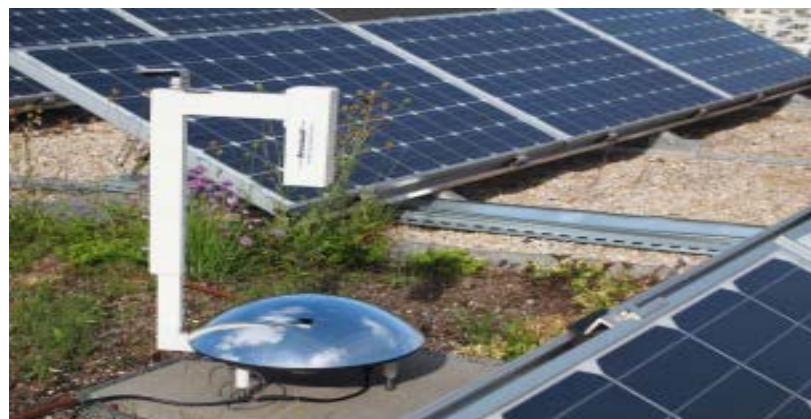
Fig 2.11 Reuniwatt InstaCast Sky Insight infrared sky imager.
