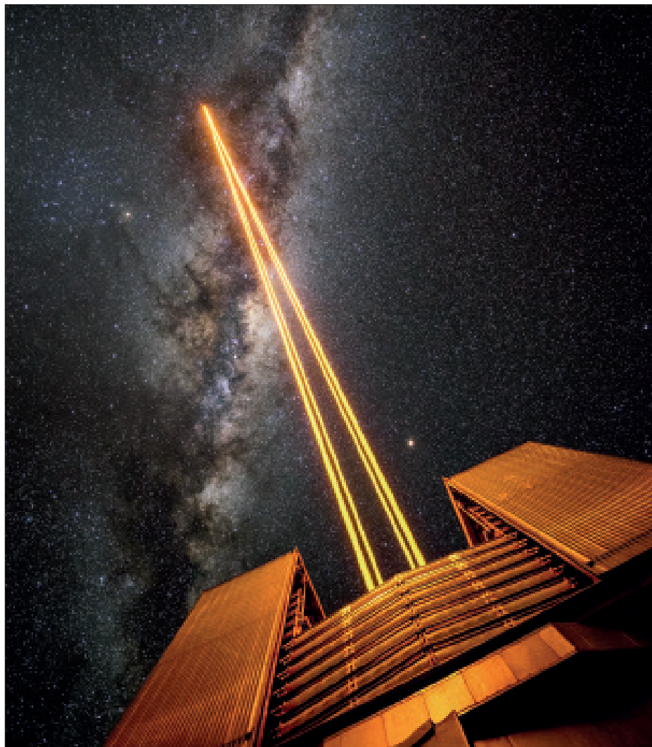
1 Four lasers create an artificial guide star from Unit Telescope 4 of ESO’s VLT at the Paranal Observatory, Chile. This is part of the VLT’s adaptive optics system, a technology which corrects the blurring effects of the Earth’s atmosphere to produce higher resolution images. (G Hüdepohl [atacamaphoto.com]/ESO)
