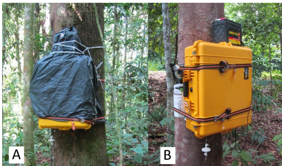
Figure 23 iDirac deployed in primary forest to measure ambient isoprene concentration A) With waterproof cover B) Without waterproof cover.
