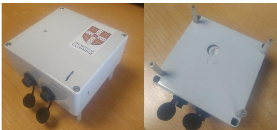
Figure 44 Image of the carbon dioxide in-house sensor showing connection ports and the underside of the sensor with the diffusion membrane and temperature sensor
