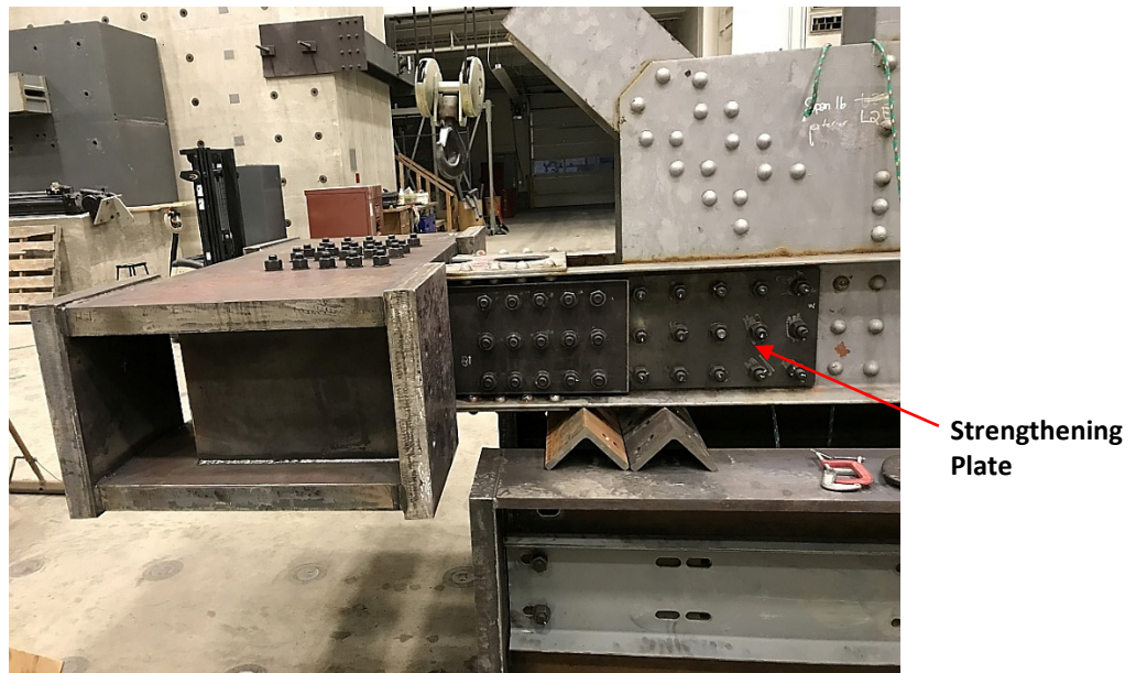
Figure 3.23. Connection at the reaction end of the specimen showing the additional plate
