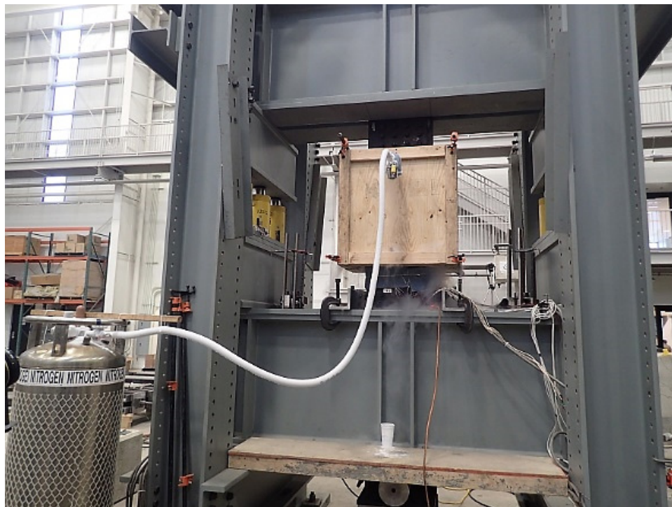
Figure 3.7 Cooling chamber used to reduce specimen toughness
