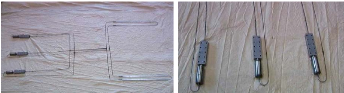
Fig. 5 Photos of “Zmey Gorynych” LHP Evaporators [9]
