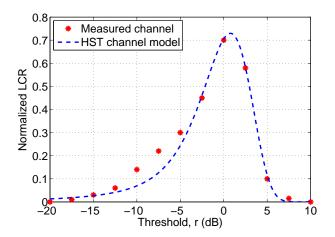
Fig. 5. The LCRs of the generic HST channel model and the measured channel in [12] in viaduct scenario ( $f_c = 930$  MHz,  $v_R = 180$  km/h, L = 15 m,  $H_{\rm viad} = 20$  m,  $H_{\rm BS} = 44$  m,  $H_{\rm MRS} = 30$  cm,  $H_{\rm train} = 3.8$  m,  $D_{BP} = 400$  m,  $\gamma_R = 0$ ,  $\beta_R = \beta_T = 60^\circ$ ,  $\mu_R^{(i)}(t_0) = 85^\circ$ ,  $k_R^{(i)} = 7.3$ , N = 50).
