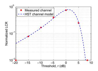
Fig. 7. The LCRs of the generic HST channel model and the measured channel in [13] in cutting scenario ( $f_c = 930$  MHz,  $v_R = 260$  km/h, L = 15 m,  $H_{\rm cut} = 7.1$  m,  $H_{\rm BS} = 28$  m,  $H_{\rm MRS} = 30$  cm,  $H_{\rm train} = 3.8$  m,  $W_{\rm up} = 53.93$  m,  $W_{\rm down} = 14.78$  m,  $D_{BP} = 200$  m,  $\gamma_R = 0, \beta_R = \beta_T = 60^\circ, \mu_R^{(i)}(t_0) = 145^\circ, k_R^{(i)} = 4, N = 50$ ).
