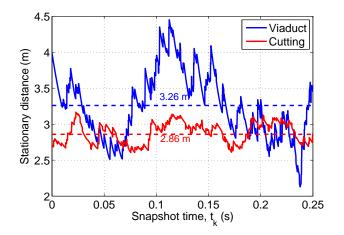
Fig. 8. The stationary distances of the generic HST channel model in viaduct and cutting scenarios (viaduct:  $f_c = 1.890$  GHz,  $v_R = 285$  km/h, L = 15 m,  $H_{\text{viad}} = 20$  m,  $H_{\text{BS}} = 20$  m,  $H_{\text{MRS}} = 30$  cm,  $H_{\text{train}} = 3.8$  m, cutting:  $f_c = 2.35$  GHz,  $v_R = 200$  km/h, L = 20 m,  $H_{\text{cut}} = 5$  m,  $H_{\text{BS}} = 28$  m,  $H_{\text{MRS}} = 30$  cm,  $H_{\text{train}} = 3.8$  m,  $W_{\text{up}} = 40$  m,  $W_{\text{down}} = 16$  m).
