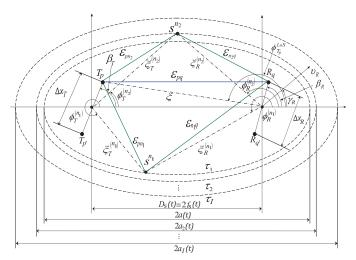
Fig. 1. The GBSM for a wideband MIMO HST channel.
