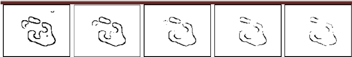
Figure 3-11 - Marr-Hildreth edges detected with \sigma=4 and spreads between 0.1 and 0.5
