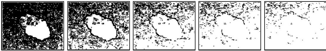
Figure 3-16 - Colour gradient edge detection with thresholds = 10, 20, 30, 40 and 50
