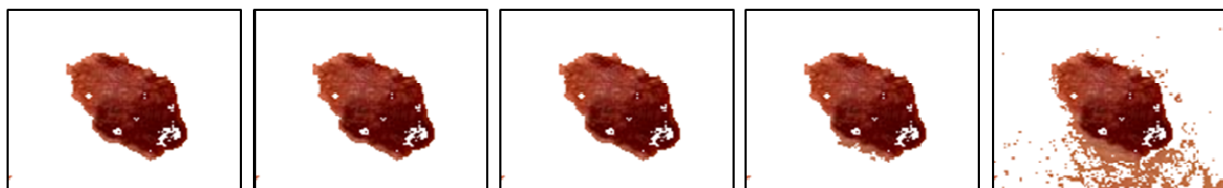
Figure 3-18 - Hue-Sat Histogram areas with Hue threshold = 70% of the maximum Hue histogram value and Sat = 40%, 50%, 60%, 70% and 80% of the maximum Saturation histogram value
