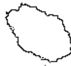
Figure 3-23 - Edge resulting from the combination of the outputs from the Sobel filter and the double thresholds
