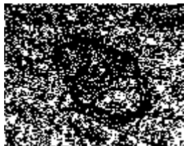
Figure 3-22 - Output of the Sobel filter applied to the smoothed grey level image
