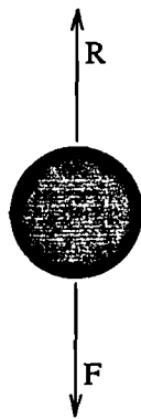
Figure 3.1 A free falling particle under the action of gravity and resistance forces
