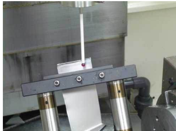
Figure 2 – Adaptively probing a compressor blade
