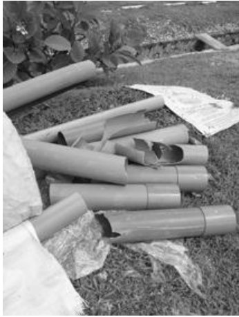
Figure 4.35: Broken PVC pipes due to incapability to support soil weight at depth below 0.6m underground. The PVC pipe buried at 0.5m is intact and remains where it is.
