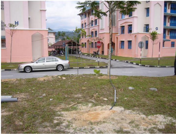
Figure 4.8: Thermocouple wires were buried underground at ground surface, 1m, 2m, 3m, 4m and 5m deep.
