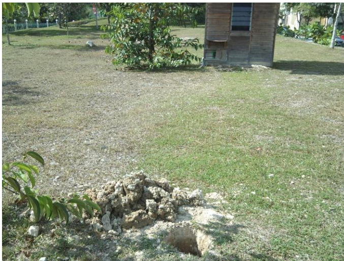
Figure 4.23: An excavated hole where the three HOBO Pendant Temp Loggers were buried at 0.5m, 1.0m and 1.5m, 0.1m away from the buried pipes (Location: International Islamic University Malaysia, Kuala Lumpur).
