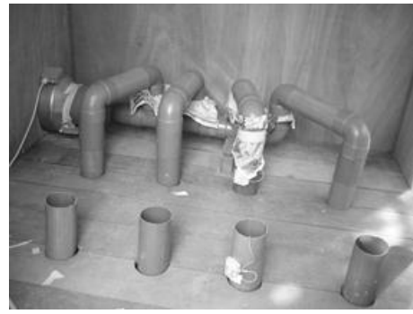
Figure 4.34: Inlets of the PVC pipes are connected to one fan blower that has three variable speeds. The fan blower extract air from outside and blow the air into the pipe inlets.
