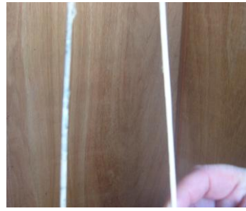
Figure 5.45: A stick used to hang data logger in PVC pipe outlet were found to be covered with mould.
