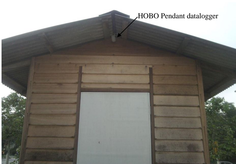
Figure 4.20: The location of HOBO Pendant Temp data logger that measured the outdoor dry bulb temperature (DBT) from March until July (Location: International Islamic University Malaysia, Kuala Lumpur).
