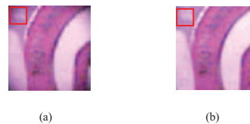
Figure 4. The flat field correction of a channel image. (a) Before the flat field correction. (b) After the flat field correction.
