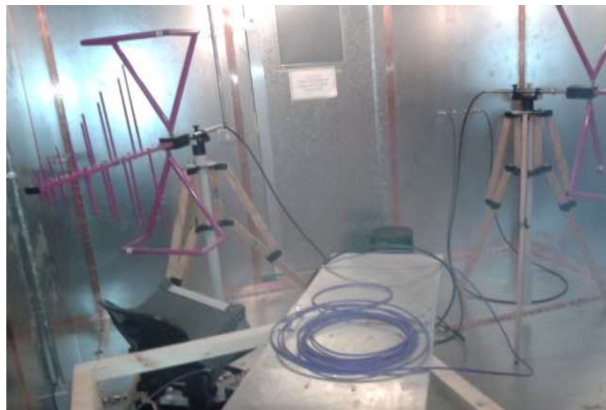
Figure 3. 4 Showing cable under test in the reverberation chamber
