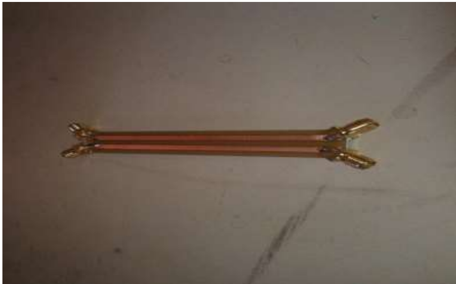
Figure 6. 2 Showing the Microstrip Symmetric/balanced test structure
