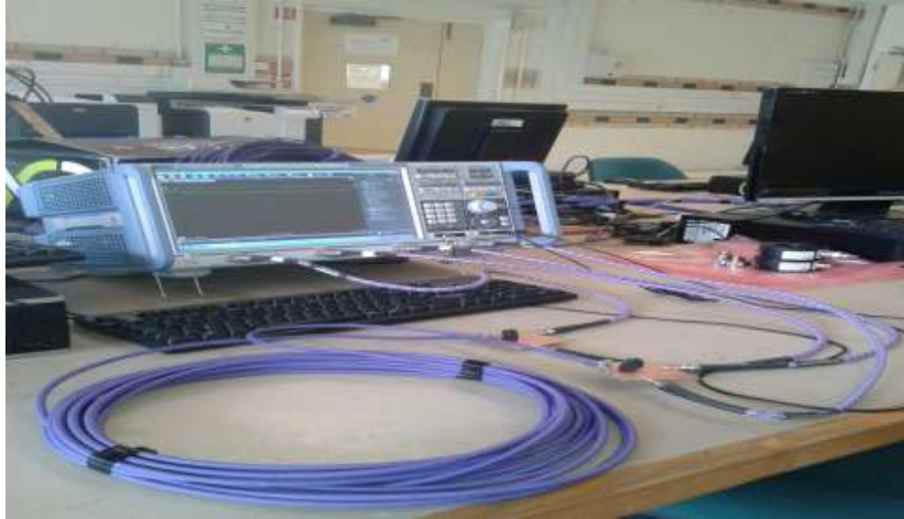
Figure 6. 15 Balanced 2-Port s-parameter testing of the 10m length of Cat 6 UTP network cable
