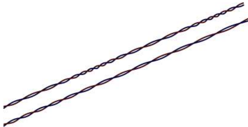
Figure 8. 1 Examples of twist nonuniformities in TWP [130]
