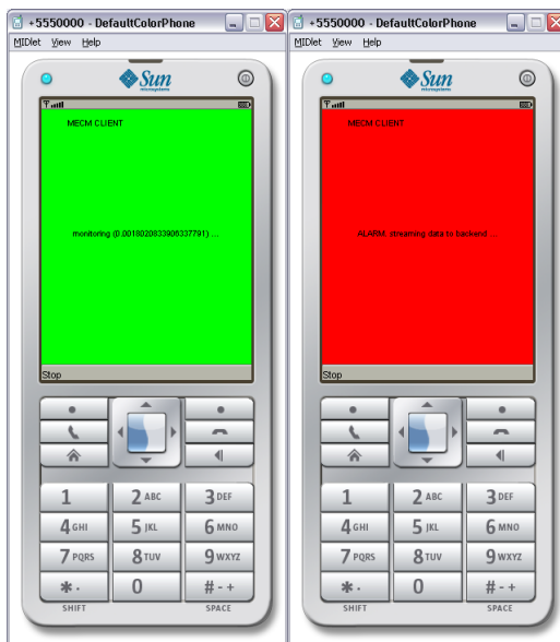
Figure 6.3: Snapshot of the mobile MECM classifier during an experiment running in the Wireless Toolkit device emulator
