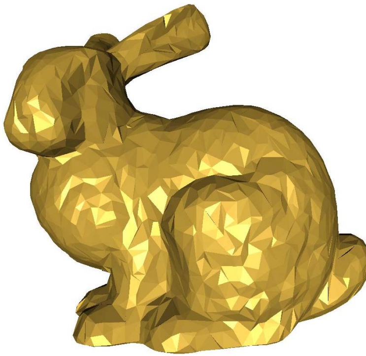
Fig. 2. Bunny model consisting of 5,597 triangles and 2,907 vertices.
