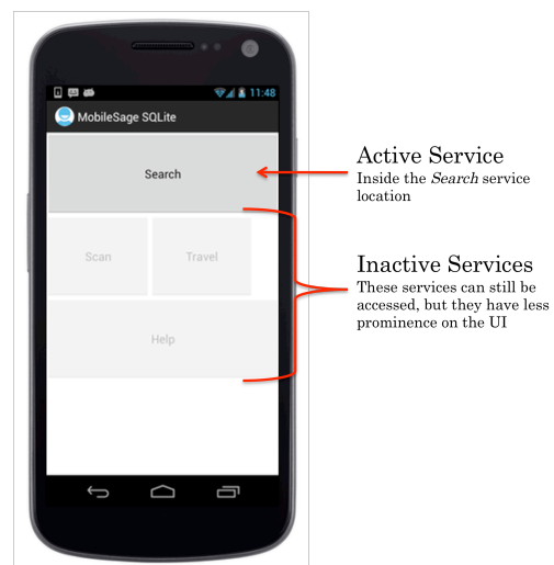
Figure 7. Screenshot of the adapted UI when the user enters a designated area around a Search centroid. Unused service
