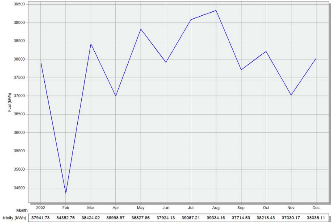
Fig. 8.11. Fuels total for a building with energy-efficient windows and ground source heat pump: first 12 storeys
