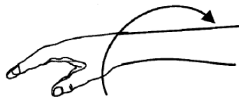
Figure.32 Supination of the forearm, used to control the cursor movement direction to relative coordinate x: - ( \rightarrow 0^\circ ) Source: ISO 9241-9 (ISO, 2000c)
