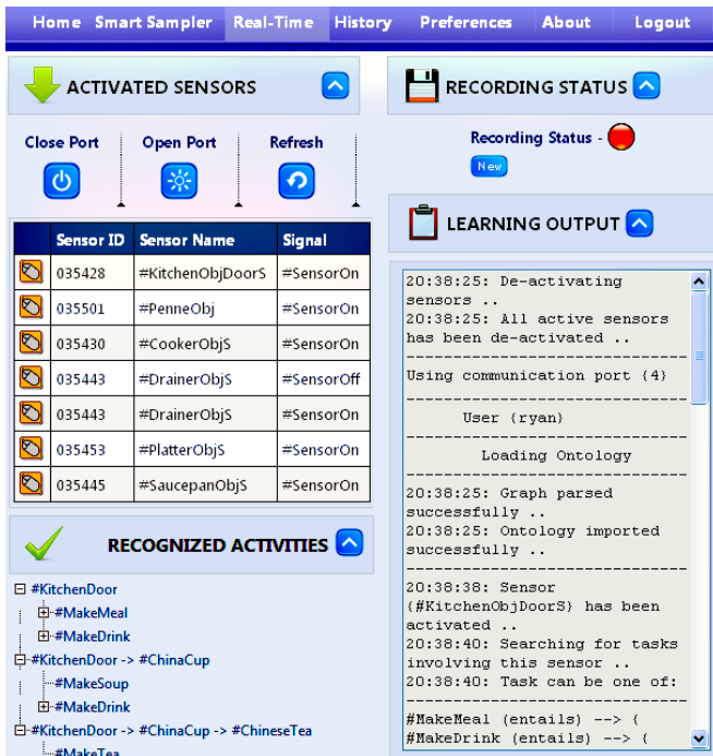
Fig. 4. The system interface operating in real time mode. In the left-hand side, the top panel is used for communication port setup; the middle panel displays the sequence of activated objects; and the bottom panel presents progressively recognized activities in a tree-like hierarchy. In the right-hand side, the top panel contains function buttons for data recording and playback; the bottom panel presents a temporal trace of events during the system operation. The system can import activity ontologies, specify reasoning and learning parameters, select the modality of audio reminder, configure hardware and define event priorities and user activity profiles.
