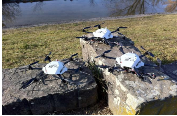
Figure 1.8 : “The three SFLY hexacopters designed for inertial-visual navigation in GPS-denied environments.” Source : (Scaramuzza, et al., 2014) – Sfly Project : www.sfly.org
