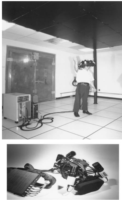
Figure 2.1 : Active Markers - Electro-optical head-tracking system (Self-Tracker) Source: (Welch, et al., 2001).
