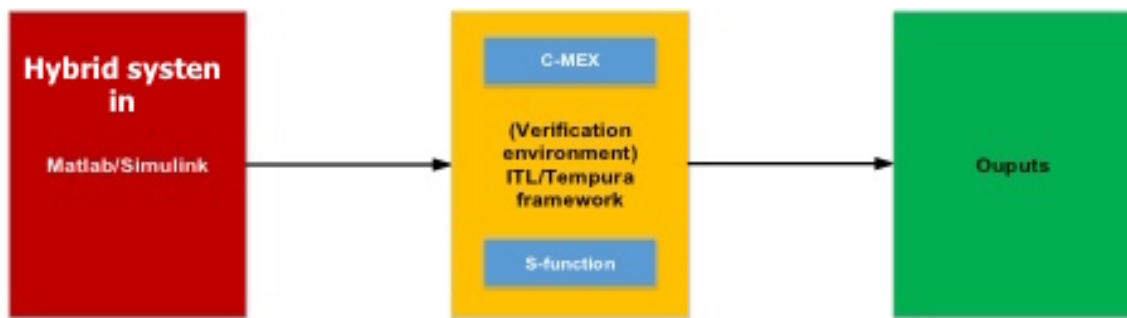
Figure 5.2: The integration of ITL/Tempura within MATLAB/Simulink using C-MEX S-function
