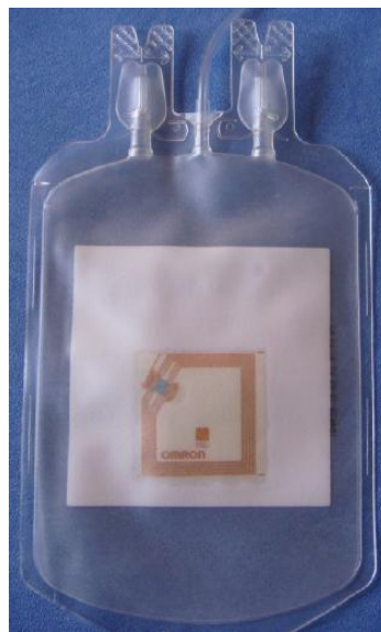
Figure 22: Ready implemented passive RFID [59]
