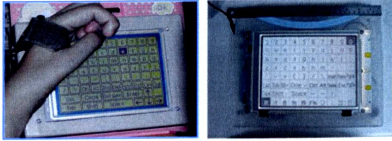
Figure 4-15 5.7 inch dimension (the left-hand side) and 9 inch dimension (the right-hand side) touchscreen input prototypes.
