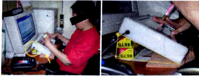
Figure 5-31 Lift the touchscreen with some rigid material to adjust the touchscreen to fit the subject's viewing angle.
