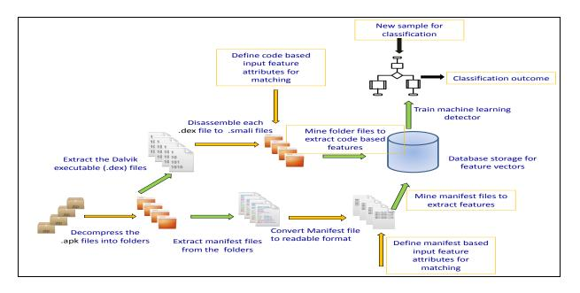
Figure 1: Custom built APK analyzer for feature extraction and classification to identify malicious Android applications.
