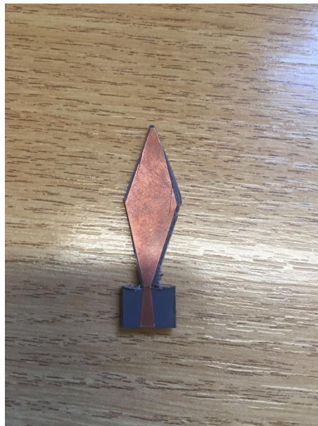
Figure 6.4: Fabricated diamond shaped antennas
