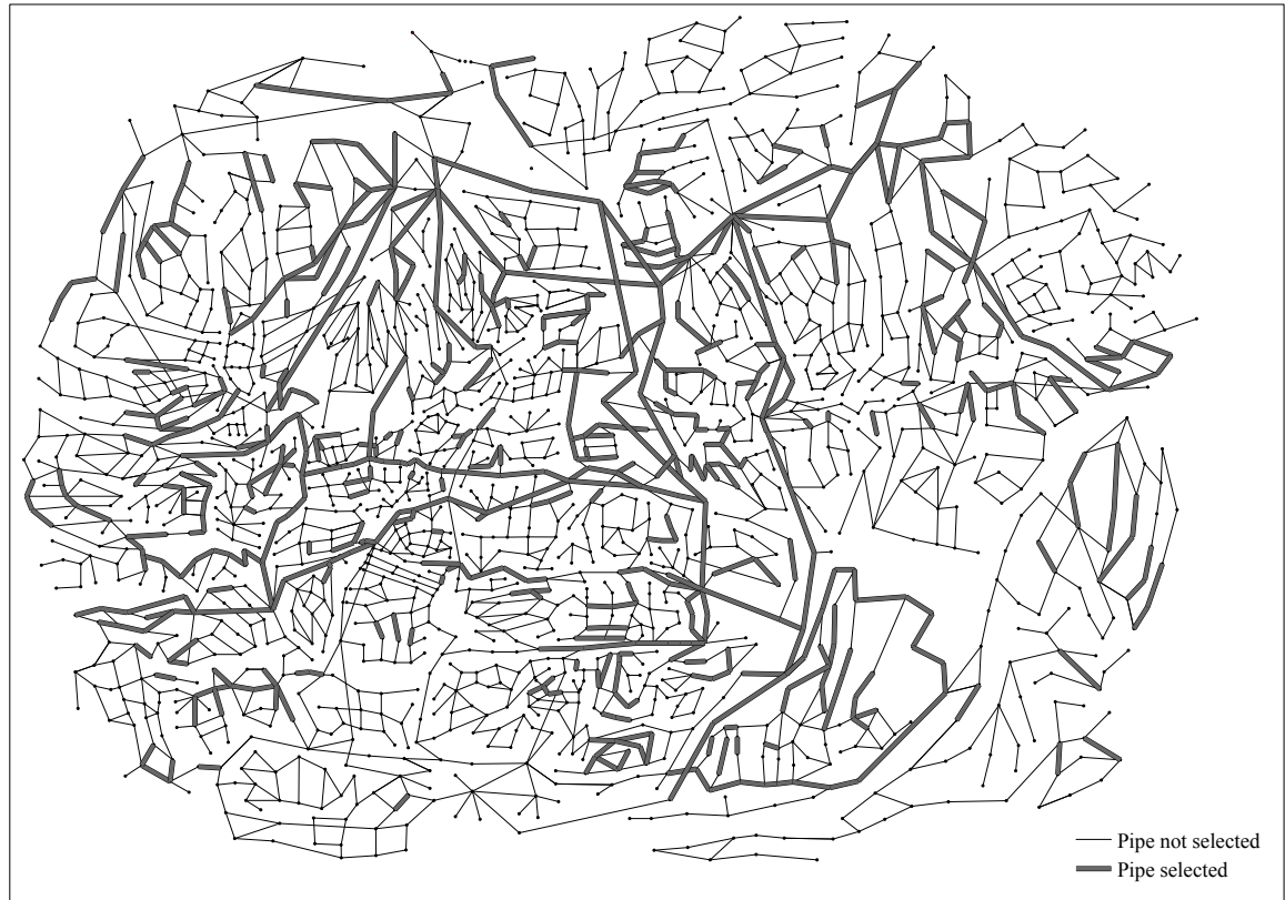
Figure 9. Pipes selected for rehabilitation based on engineering judgement
