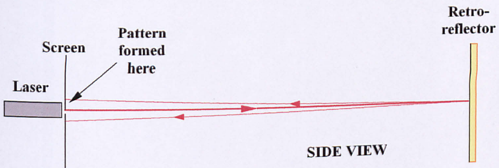
(a) Reflection Pattern Test Set-up
