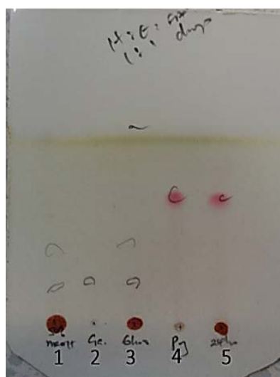
Figure 4. 12: TLC chromatogram showing the presence of gallic acid in both 50% aqueous methanol and six hours extract whereas pyrogallol was only present in 24hours extract. Where 1 = 24 hours 50% methanol aqueous extract, 2 = gallic acid, 3 = 6 hours aqueous extract, 4 = pyrogallol and 5 = 24 hours aqueous extract
