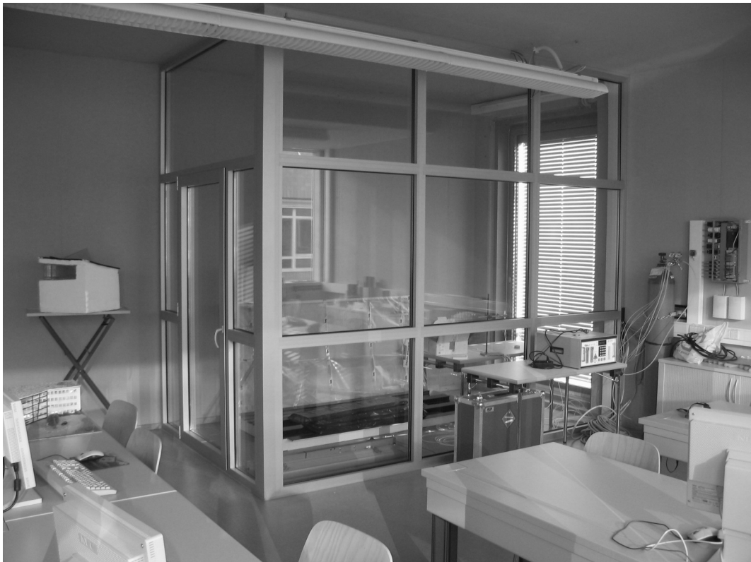
Figure E.1: Photograph showing the Labor für Gebäudesimulation G1.02 (laboratory room) with the glass compartment in the corner of the room at the beginning of the project. Originally, the glass compartment was intended to be used as a test facility for façade elements. Then, the experimental chamber for this work was constructed within this glass compartment as can be seen in subsequent photographs.
