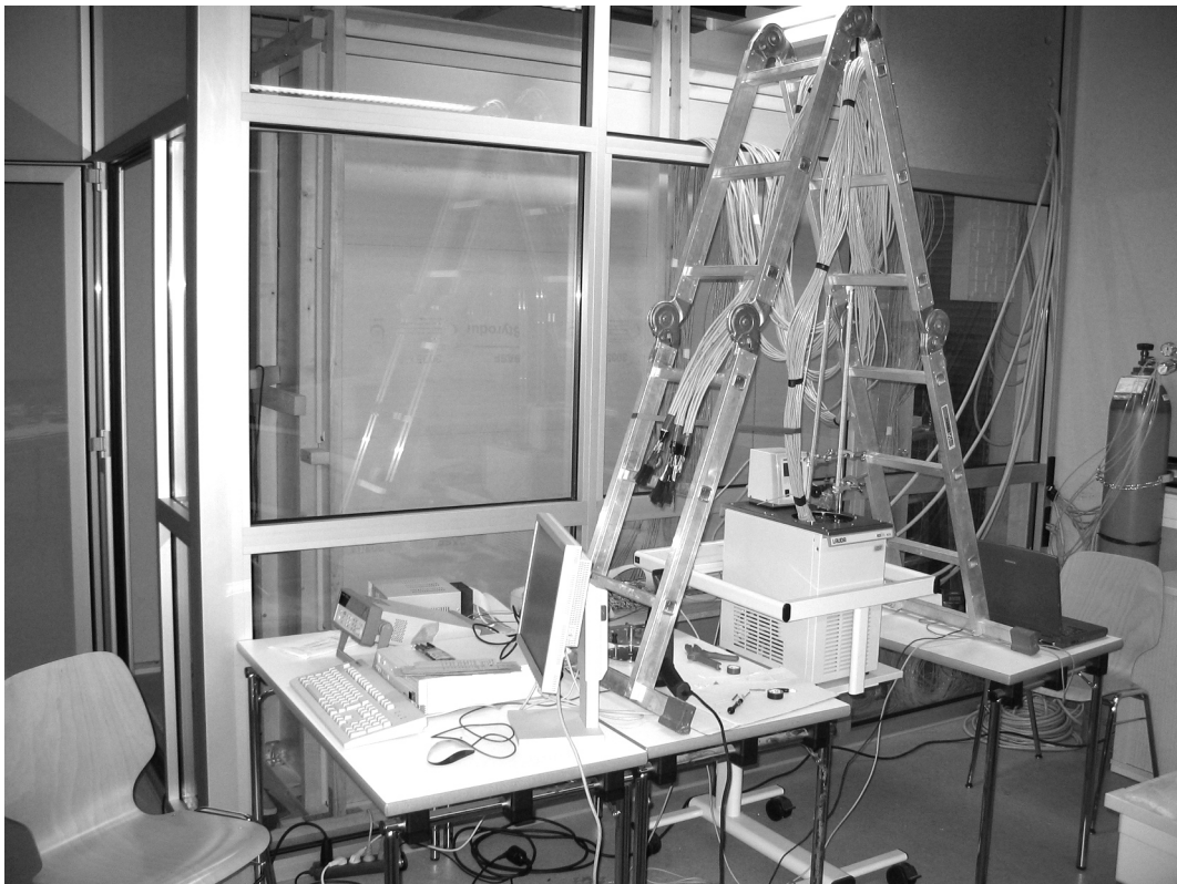
Figure E.6: Photograph showing the newly built chamber inside the glass compartment. In the front, temperature sensors are being calibrated before getting installed inside the chamber.
