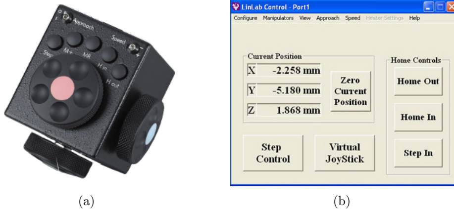
Figure 3.6: (a) Scientifica's micro-manipulator controller and (b) Scientifica's LinLab software [64].
