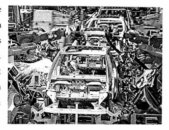
Pneumatic components are required not only to fix components into place but also to prevent these from being deformed. In daily operation, they are subjected to severe loads, both in terms of the forces present and the welding splashes falling onto their outer surfaces. As bodywork components are transported from one welding station to the next, pneumatics are used to hold and grip these. This calls for optimised individual solutions.
