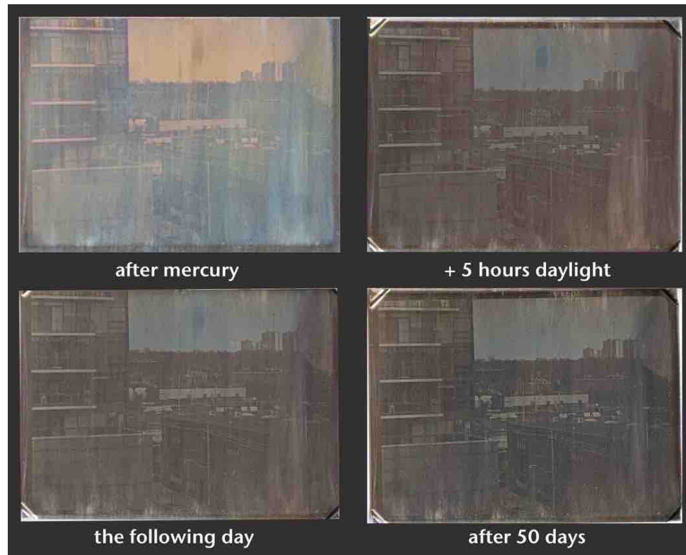
Figure 83. DagTest 11-27-2014. Mercury developed latent image highlights with silver iodide printed-out shadows.
