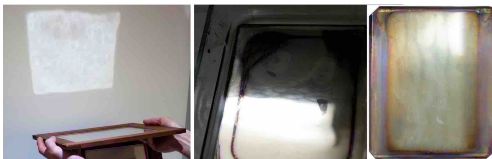
Figure 19. Planishing hammer marks visible by reflection (left), under water (centre) and half shadow-illumination right). 1840 plate on the left, others date to ca. 1853.
