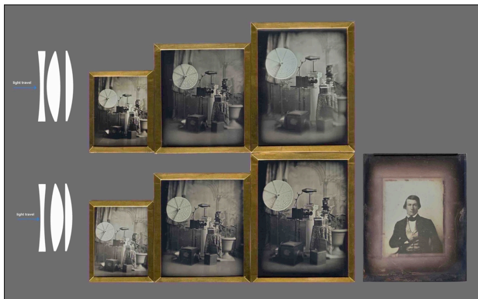
Figure 72. DagTest 11-24-2013. Daguerreotypes taken with the William H. Butler camera. Three sizes with centre element transposed incorrectly (top). Three sizes with the correct orientation for the centre element (bottom). Portrait of a man on quarter-sized plate masked to conceal spherical aberration. National Gallery of Canada, LFA. 21500_186_83 (right).
