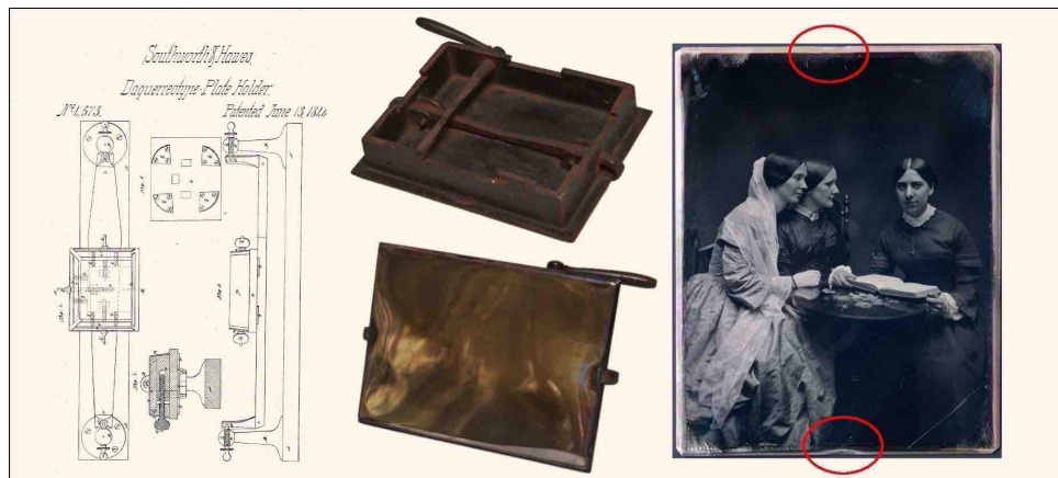
Figure 24. US Patent 4,573 dated June 13, 1846 (left). Verso and recto of the half-plate polishing block (centre). National Gallery of Canada collection, LFA 21500_601_5. Southworth and Hawes half-plate daguerreotype of three women. The plate has deformed edges due to the clamping system (right). Collection Michael Mattis and Judith Hochberg.
