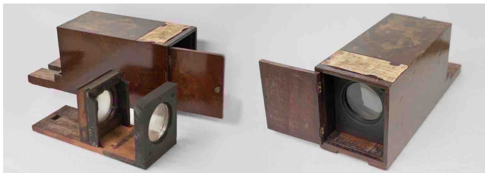
Figure 69. John Draper's experimental lens camera apart and assembled. National Museum of American History, Smithsonian. Accession number 72.072A.08. Author photograph.
