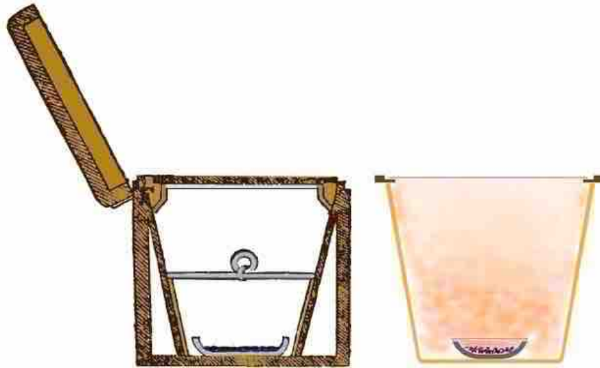
Figure 42. Iodine box enhanced cross section, from History and Practice of Photogenic Drawing , 1839, Plate II (left). Illustration of vapour distribution (right).
