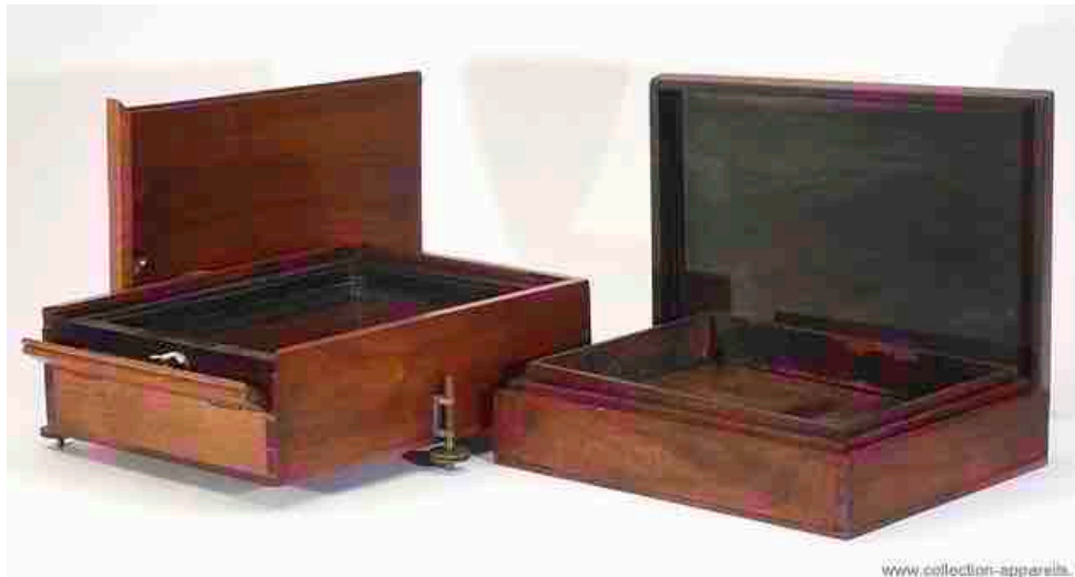
Figure 55. Foucault's design sensitizing box for bromine water (left). Iodine box incorporating an absorbent card after Séguier's design (right). Source, www.collection-appareils.fr
