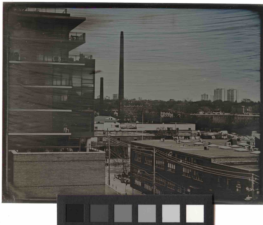
Figure 22. Dag Test 5-14-2016. Daguerreotype polished with tripoli (rottenstone) according to Daguerre's improved method from October 1839. The plate was polished with linear strokes and no acid was applied after heating the plate.
