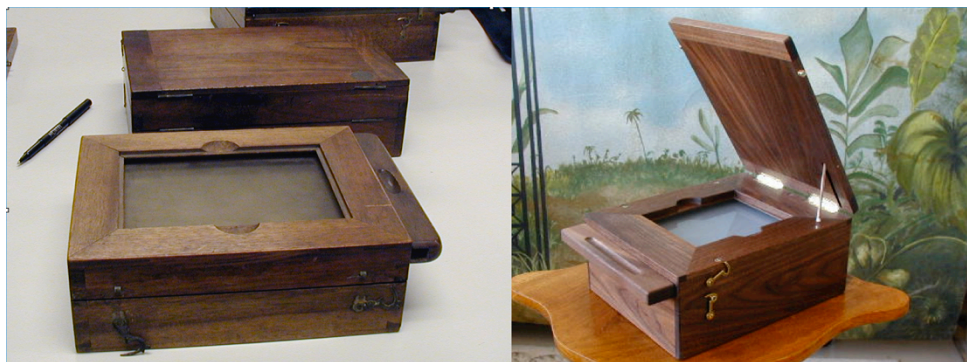
Figure 6. Nineteenth century French style sensitizing boxes (left). Author photo – GEM collection . New reproduction sensitizing box (right).
