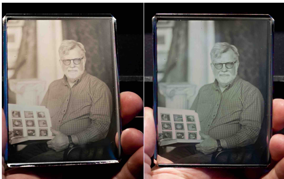
Figure 1. Dag Test 3-9-2014. Portrait of Keith F. Davis. Illustration of prismatic effect with a slight change of viewing angle appearing magenta (left) and cyan (right).
