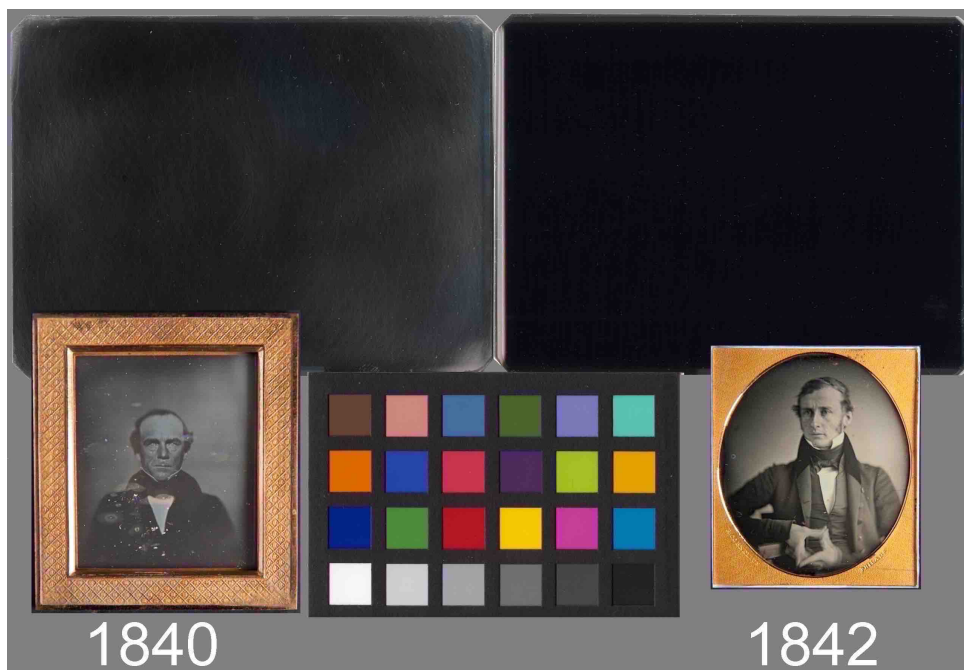
Figure 23. Modern plates polished circular with pumice (left). Linear polish with rouge (right). Overlay, Daguerreotypes by Robert Cornelius with circular polish (left), and linear polish (right).
