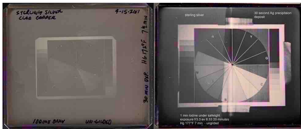
Figure 14. Dag Test 4-15-2011. Image on sterling silver clad plate (left). Dag Test 3-18-2012. Sterling plate with pure silver deposited on right side before use (right).
