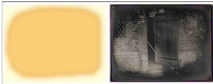
Figure 45. Iodine coating simulation (left). The Open Door , daguerreotype, 2012 showing the effect of light iodine coatings on the perimeter (right).
