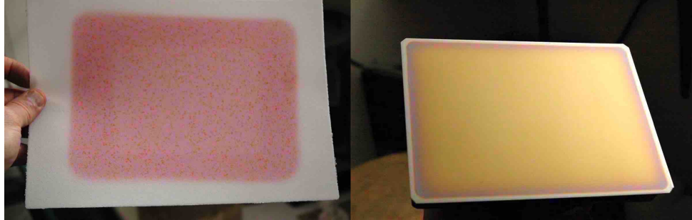
Figure 44. Iodine absorbed porous plastic panel (left). Iodized silver plate (right).
