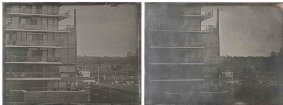
Figure 15. Dag Test 3-13-2013. Image on fine silver (left). Image on sterling silver (right).
