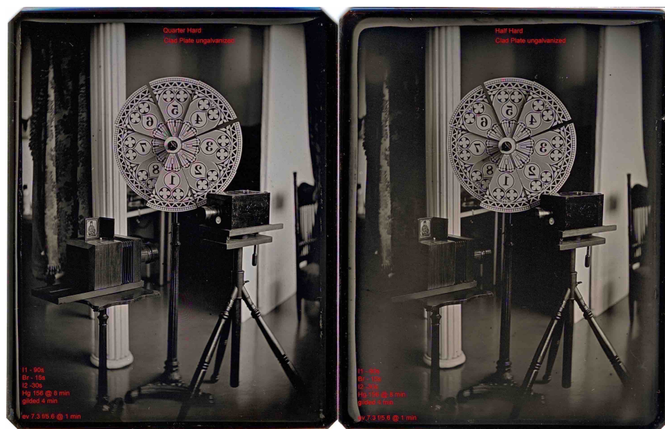
Figure 5. Daguerreotype on a quarter-hard plate (left), and identically prepared example on a half-hard plate (right).
