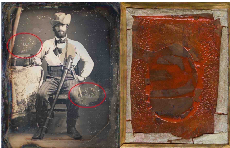
Figure 25. Daguerreotype of a surveyor with copper sulphate corrosion due to porous silver (left). Verso of the plate indicating that it was not galvanized. Note the red wax used to adhere the plate to a wooden block for buffing (right). Collection of Lawrence T. Jones.
