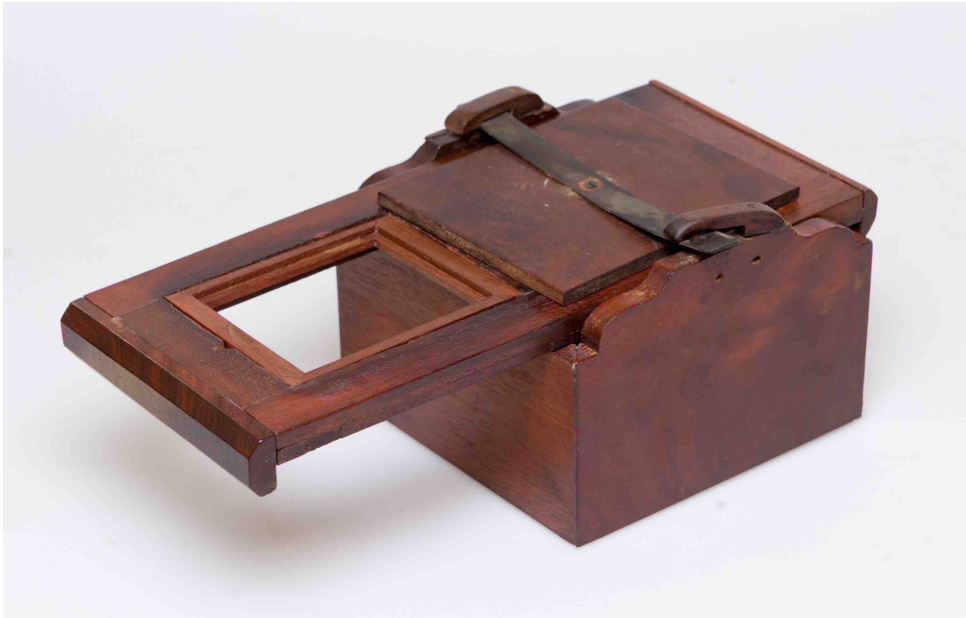
Figure 46. Iodine coating box built by John Roach. National Gallery of Canada collection. LFA 21500_601_31.
