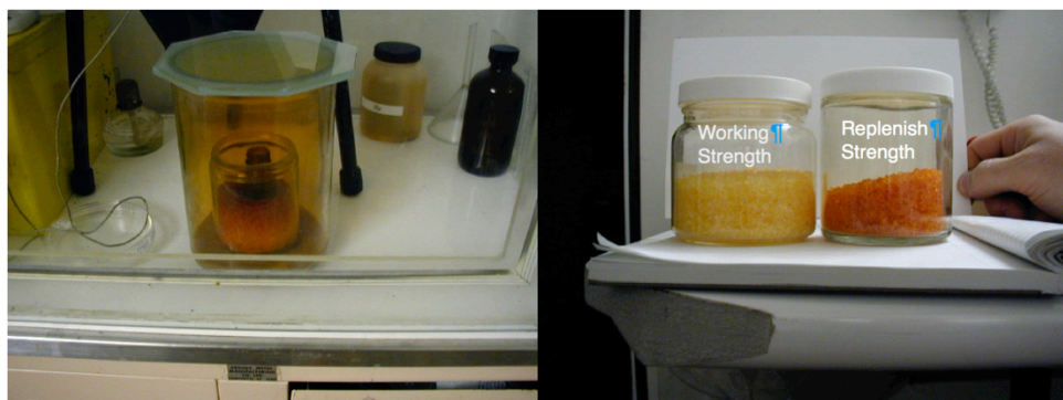
Figure 7. Bromine vapour absorbed by silica gel (left). The concentration of bromine is judged by colour. Working strength gel appears yellow, replenish strength gel appears red-orange (right).
