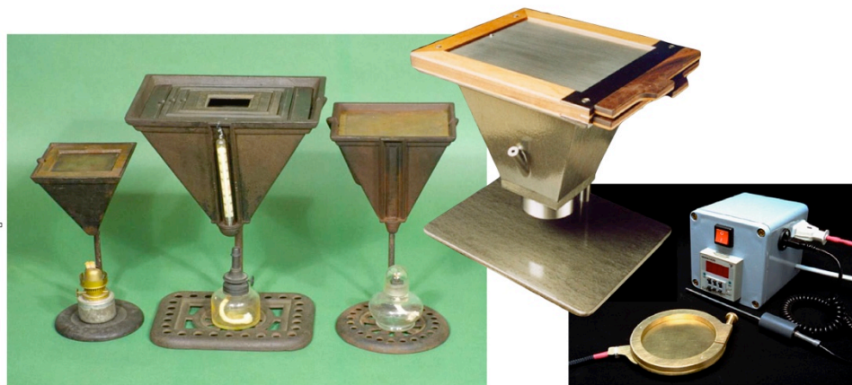
Figure 9. Nineteenth century cast iron mercury baths in quarter, full and half-plate size. Heating is done with an alcohol lamp (left). National Gallery of Canada collection. Modern mercury bath with improvements including an automated mercury temperature controller (right).
