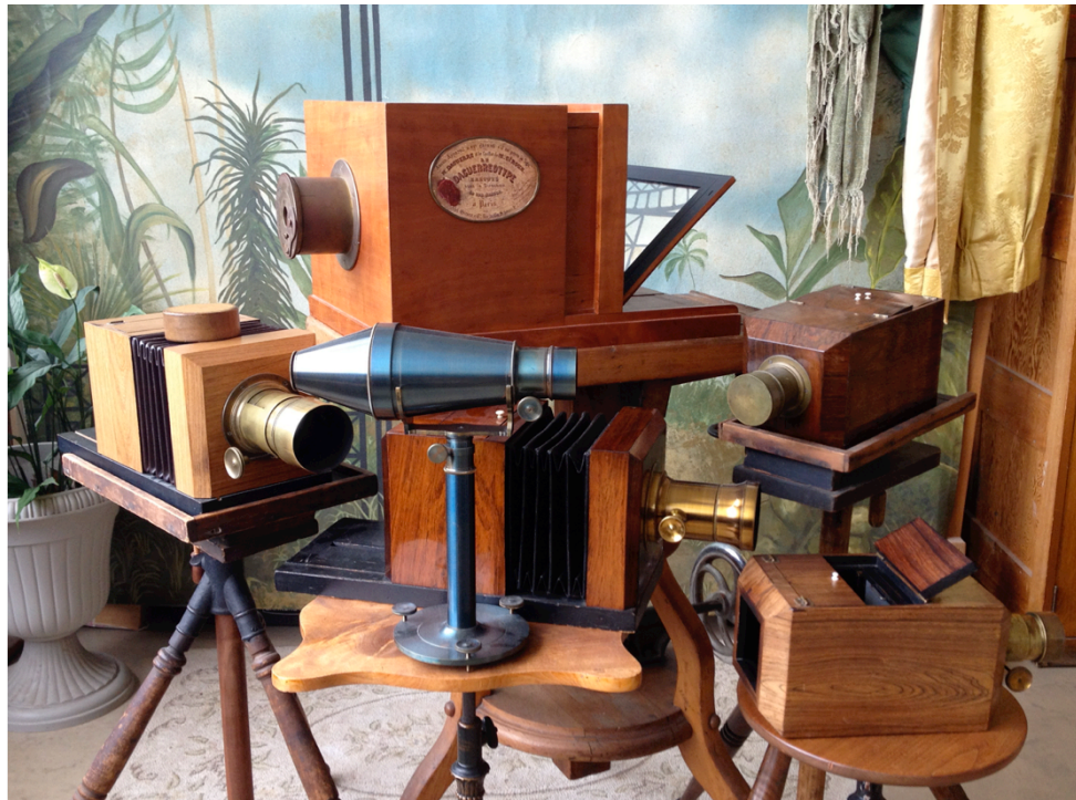
Figure 8. Clockwise from the left, a replica half-plate Palmer and Longking camera with Voigtländer lens, a full-plate replica of Daguerre's camera with landscape achromatic lens, an original L.B.B. & Co. quarter-plate chamfered box camera and lens, ca 1843, a replica quarter-plate chamfered box camera with Voigtländer lens, an original half-plate Palmer and Longking camera with C.C. Harrison lens, and a replica Voigtländer all-metal camera for taking round daguerreotypes.
