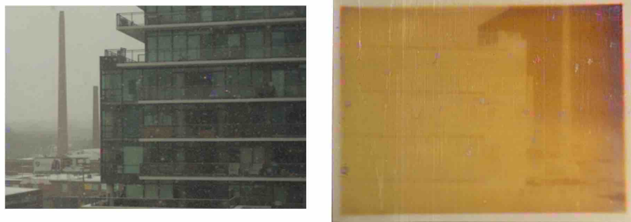
Figure 34. DagTest 2-16-2013. View from studio window (left). In camera, unfixated silver iodide print-out negative (right).
