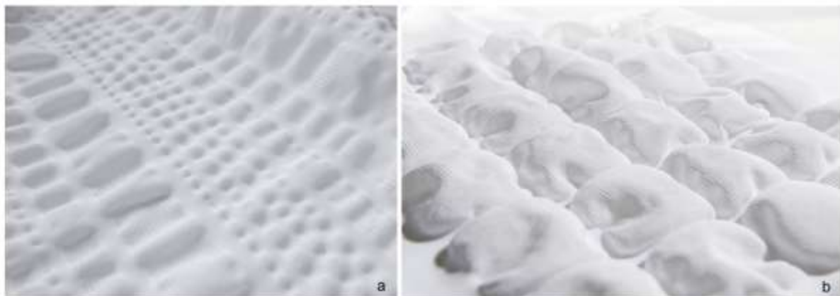
Figure 8. a) Seer sucker effects achieved by tension applied to one axis. b) Full shapes achieved by even bi-axial tension © Laura Morgan 2016
