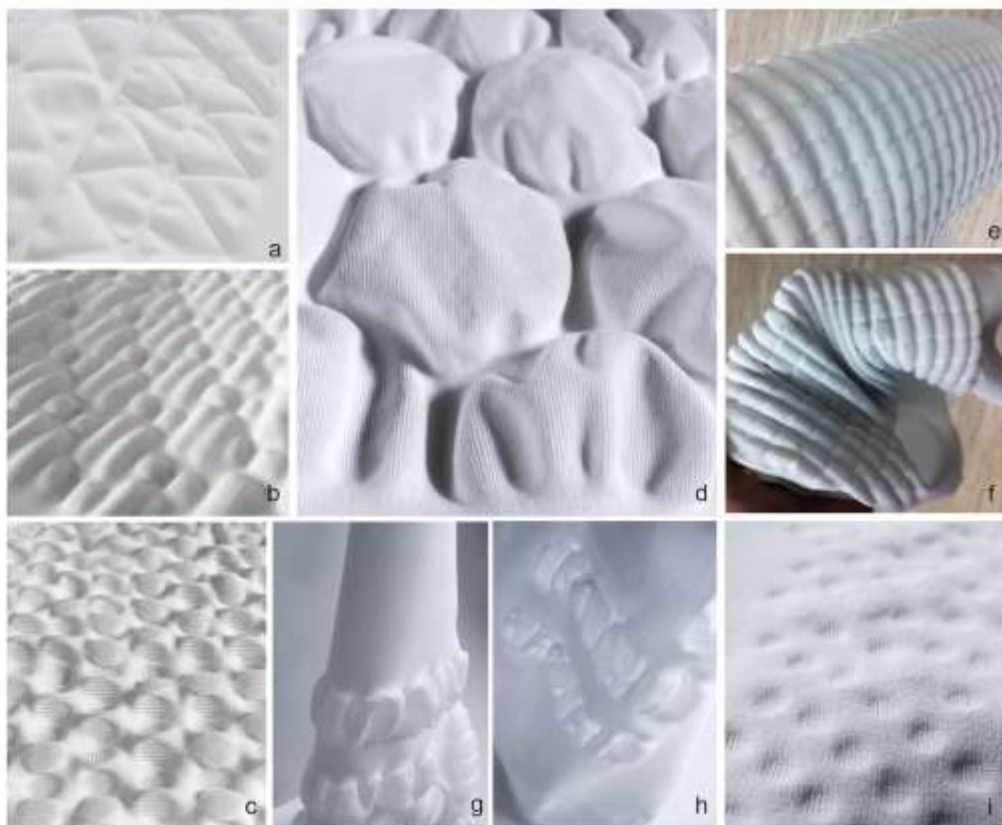
Figure 11. Laser moulded design samples inspired by traditional textile constructions: a) quilted effects; b) basket weave; c) honeycomb; d) large moulded forms; e- f) pleated effects; g-h) gathering effects; i) small scale dimpled effects © Laura Morgan 2016
