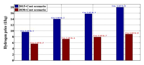
Figure 9.16: Central alkaline electrolyser hydrogen price for different cost scenarios and under different system sizes
