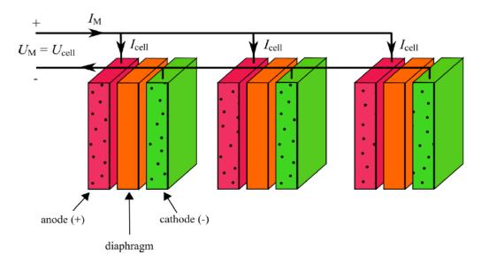
Figure 4.2: Monopolar cell arrangement(Carmo et al., 2013)
