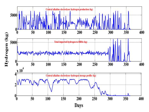
Figure 9.13: Central hydrogen production, hydrogen imported at HRSs and central storage profile (6,410 kg/day alkaline central electrolyser under 2015-Cost scenario (Cen. LAE Sc. 4))
