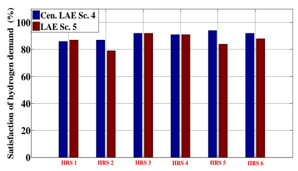
Figure 10.7: Comparison of Triple-default electrolyser size (LAE Sc. 5) and 6,410 kg/day alkaline central electrolyser without electrolyser at the HRSs (Cen. LAE Sc. 4)
