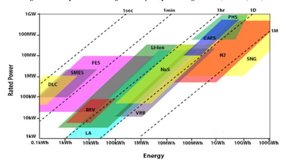
Figure 2.11: Comparison of capacity of rated energy vs. rated power with period of discharge for ESSs.
