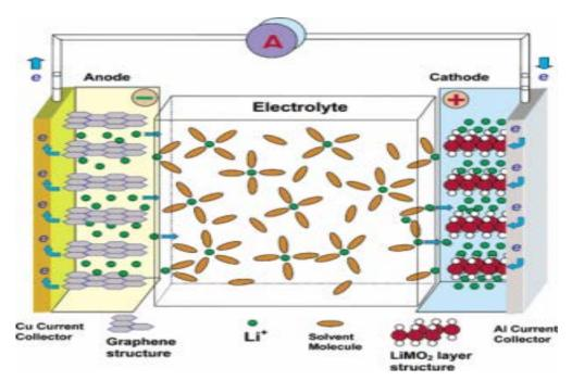
Figure 2.6: Schematic diagram of a Li-ion battery
