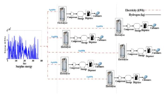
Figure 7.14: Overall system in Off-peak only scenario (2015-Cost scenario)
