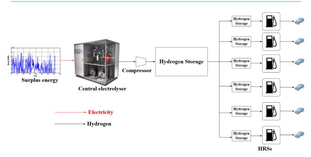
Figure 9.1: Summary of the system process when central electrolyser is applied without forecourt electrolysis
