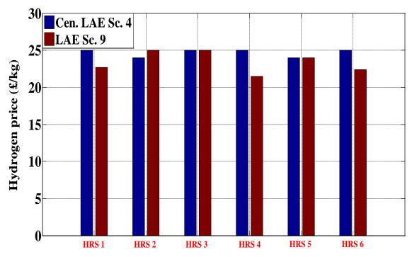
Figure 10.15: Comparison of Combination of HRSs and 4,853 kg/day alkaline central electrolysers (LAE Sc. 9) and 6,410 kg/day alkaline central electrolyser without electrolyser at the HRSs (Cen. LAE Sc. 4)
