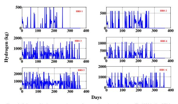
Figure 9.18: Imported hydrogen at each garage forecourt throughout the year profile (2383 kg/day PEM central electrolyser (Cen. PEME Sc. 1)) under 2015-Cost scenario
