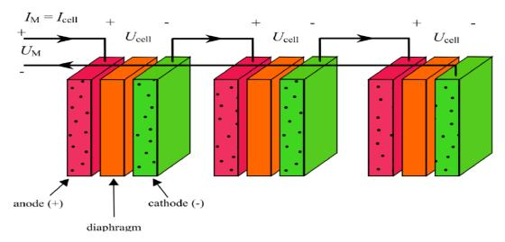
Figure 4.3: Bipolar cell arrangement(Carmo et al., 2013)
