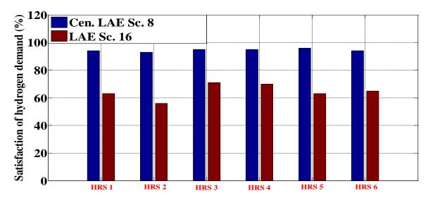
Figure 10.17: Comparison of Only onsite alkaline electrolyser without central electrolyser (LAE Sc. 16) and 6,410 kg/day alkaline central electrolyser without electrolyser at the HRSs (Cen. LAE Sc. 8)
