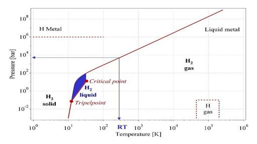
Figure 3.5: Diagram of hydrogen phase
