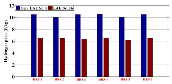
Figure 10.20: Comparison of Only onsite alkaline electrolyser without central electrolyser (LAE Sc. 16) and 6410 kg/day alkaline central electrolyser without electrolyser at the HRSs (Cen. LAE Sc. 8)
