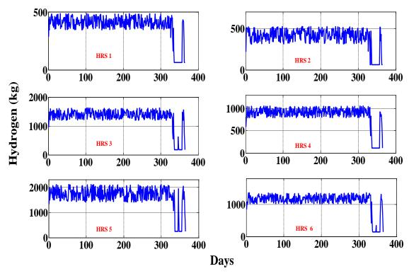
Figure 9.31: Daily variation of hydrogen level in storage tank throughout the year (6410 kg/day PEM central electrolyser (Cen. PEME Sc. 8)) under 2030-Cost scenario
