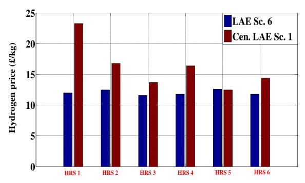
Figure 10.14: Comparison of Combination of HRSs and 1,098 kg/day alkaline central electrolysers (LAE Sc. 6) and 2,383 kg/day alkaline central electrolyser without electrolyser at the HRSs (Cen. LAE Sc. 1)
