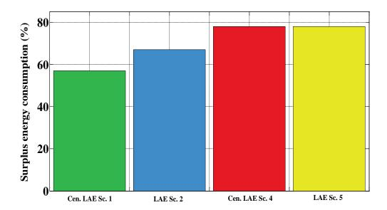
Figure 10.8: Energy consumption of Double-sized default electrolyser size (LAE Sc. 2) ,Triple-sized default electrolyser (LAE Sc. 5) , 2,383 kg/day (Cen. LAE Sc. 1) and 6,410 kg/day (Cen. LAE Sc. 4) alkaline central electrolysers without electrolyser at the HRSs
