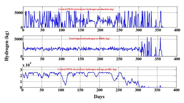
Figure 9.26: Central hydrogen production, hydrogen imported at HRSs and central storage profile (5,495 kg/day PEM central electrolyser (Cen. PEME Sc. 7)) under 2030-Cost scenario
