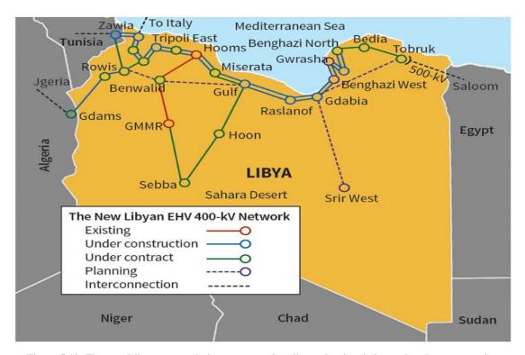
Figure 5.12: The new Libyan transmission system and outlines what is existing and under construction (Daloub, 2017)
