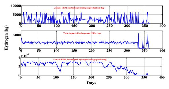
Figure 9.29: Central hydrogen production, hydrogen imported at HRSs and central storage profile (6410 kg/day PEM central electrolyser (Cen. PEME Sc. 8)) under 2030-Cost scenario
