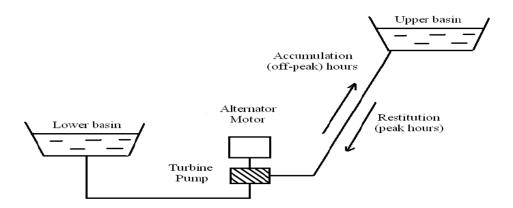
Figure 2.2: Illustration of the PHES process
