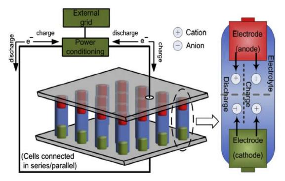
Figure 2.5: Battery energy storage system operation
