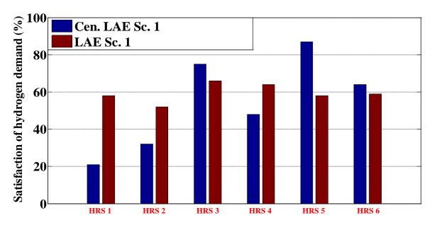
Figure 10.1: Comparison of Only onsite alkaline electrolyser without central electrolyser (LAE Sc. 1) and 2383 kg/day alkaline central electrolyser without electrolyser at the HRSs (Cen. LAE Sc. 1)
