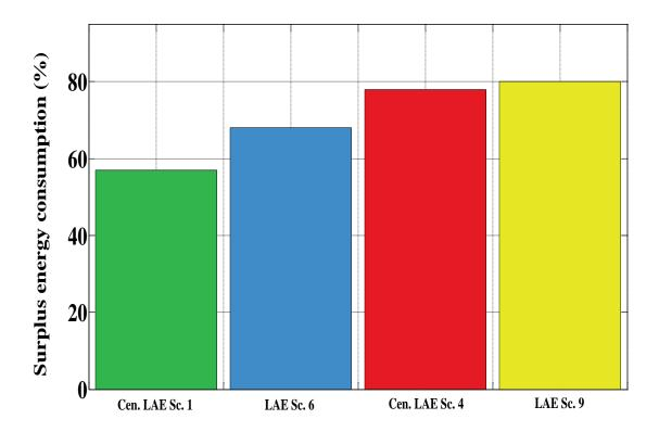
Figure 10.13: Total energy consumed in each hydrogen production scenario (alkaline, 2015-Cost scenario)
