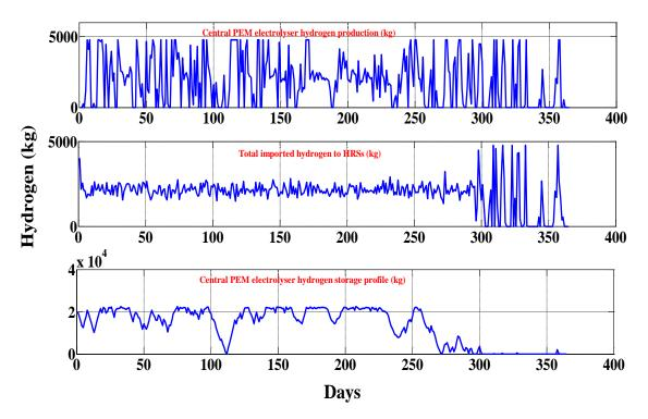
Figure 9.23: Central hydrogen production, hydrogen imported at HRSs and central storage profile (4,766 kg/day PEM central electrolyser (Cen. PEME Sc. 6)) under 2030-Cost scenario
