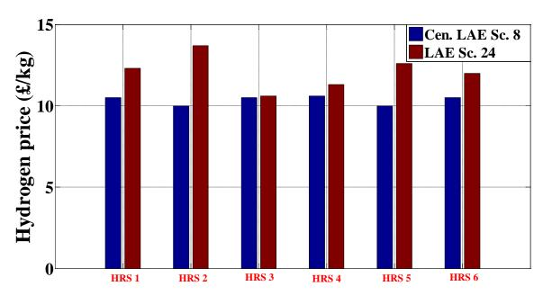
Figure 10.30: Comparison of Combination of HRSs and 4,853 kg/day alkaline central electrolysers (LAE Sc. 24) and 6,410 kg/day alkaline central electrolyser without electrolyser at the HRSs (Cen. LAE Sc. 8)
