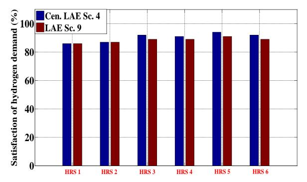
Figure 10.12: Comparison of Combination of HRSs and 4853 kg/day alkaline central electrolysers (LAE Sc. 9) and 6410 kg/day alkaline central electrolyser without electrolyser at the HRSs (Cen. LAE Sc. 4)
