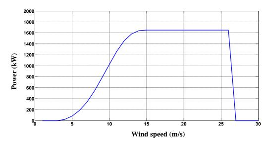
Figure 6.7: Wind turbine power curve with wind speed.
