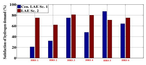
Figure 10.6: Comparison of Double-sized default electrolyser size (LAE Sc. 2) and 2383 kg/day alkaline central electrolyser without electrolyser at the HRSs (Cen. LAE Sc. 1)
