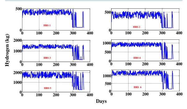
Figure 9.15: Daily variation of hydrogen level in storage tank throughout the year (6410 kg/day alkaline central electrolyser under 2015-Cost scenario (Cen. LAE Sc. 4))
