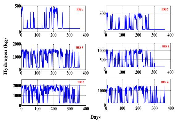
Figure 9.22: Daily variation of hydrogen level in storage tank throughout the (2,383 kg/day PEM central electrolyser (Cen. PEME Sc. 5)) under 2030-Cost scenario
