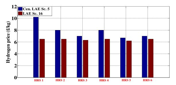
Figure 10.19: Comparison of Only onsite alkaline electrolyser without central electrolyser (LAE Sc. 16) and 2383 kg/day alkaline central electrolyser without electrolyser at the HRSs (Cen. LAE Sc. 5)
