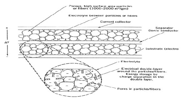
Figure 2.7: Double layer supercapacitors
