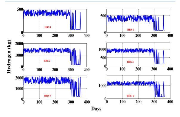
Figure 9.25: Daily variation of hydrogen level in storage tank throughout the year (4,766 kg/day PEM central electrolyser (Cen. PEME Sc. 6)) under 2030-Cost scenario
