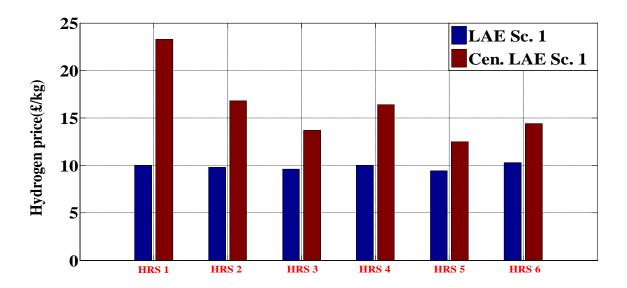
Figure 10.4: Comparison of Only onsite alkaline electrolyser without central electrolyser (LAE Sc. 1) and 2,383 kg/day alkaline central electrolyser without electrolyser at the HRSs (Cen. LAE Sc. 1)
