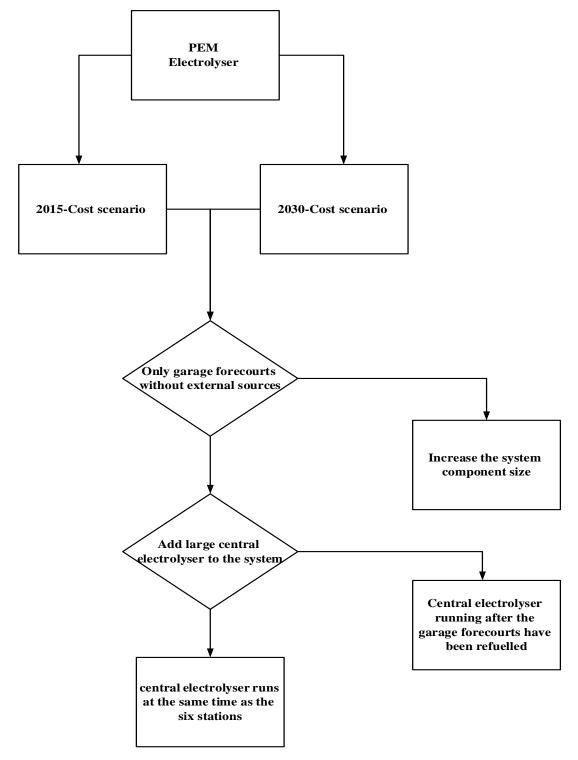
Figure 8.58: summary of the operation scenarios for PEM electrolyser under 2015 and 2030-Cost scenario
