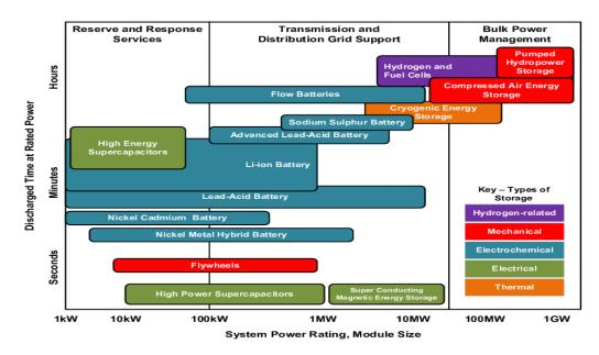
Figure 2.10: Comparison of discharge time vs. system power rating for ESSs (Luo et al., 2015).
