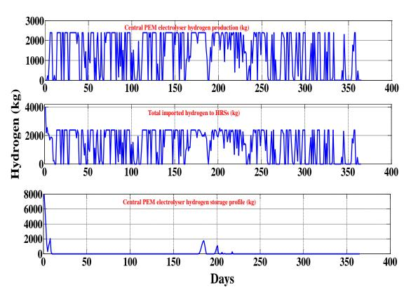
Figure 9.17: Central hydrogen production, hydrogen imported at HRSs and central storage profile (2383 kg/day PEM central electrolyser (Cen. PEME Sc. 1)) under 2015-Cost scenario
