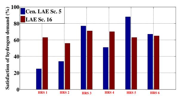
Figure 10.16: Comparison of Only onsite alkaline electrolyser without central electrolyser (LAE Sc. 16) and 2,383 kg/day alkaline central electrolyser without electrolyser at the HRSs (Cen. LAE Sc. 5)
