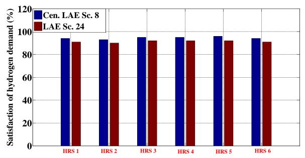
Figure 10.27: Comparison of Combination of HRSs and 4,853 kg/day alkaline central electrolysers (LAE Sc. 24) and 6,410 kg/day alkaline central electrolyser without electrolyser at the HRSs (Cen. LAE Sc. 8)
