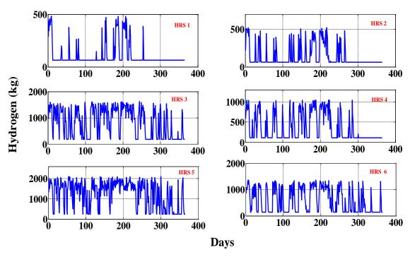
Figure 9.19: Daily variation of hydrogen level in storage tank throughout the year profile (2383 kg/day PEM central electrolyser (Cen. PEME Sc. 1)) under 2015-Cost scenario
