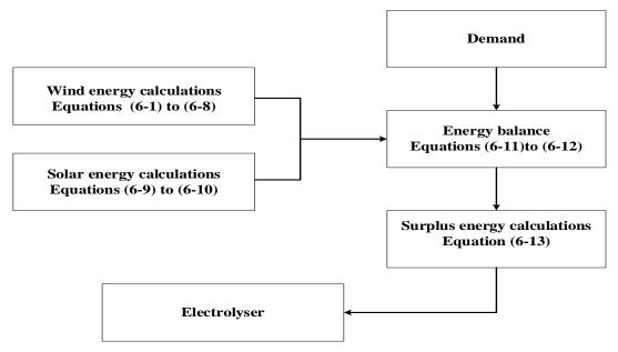
Figure 6.14: Proposed sizing system steps
