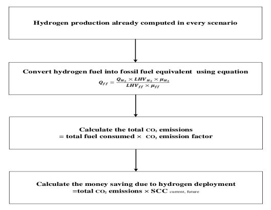
Figure 9.33: Process of saving money due to hydrogen energy penetration
