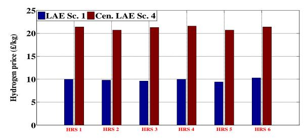
Figure 10.5: Comparison of Only onsite alkaline electrolyser without central electrolyser (LAE Sc. 1) and 6,410 kg/day alkaline central electrolyser without electrolyser at the HRSs (Cen. LAE Sc. 4)
