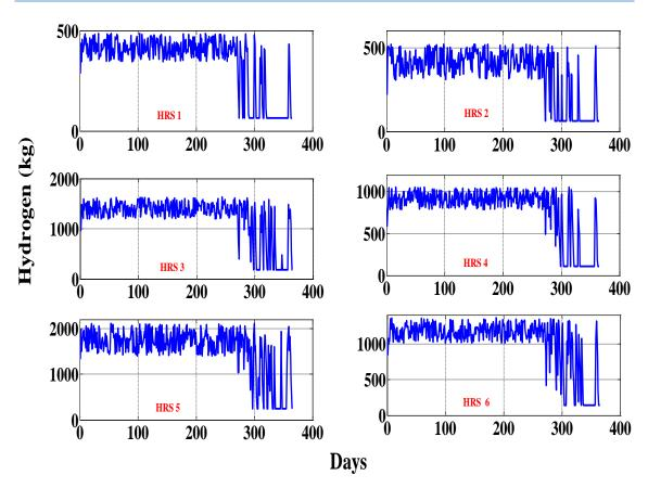
Figure 9.12: Daily variation of hydrogen level in storage tank throughout the year (5,495 kg/day alkaline central electrolyser under 2015-Cost scenario (Cen. LAE Sc. 3))
