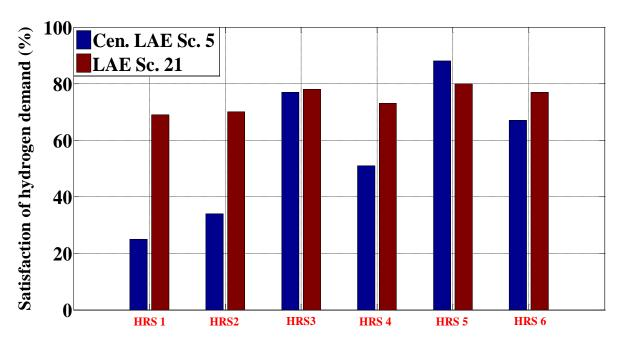
Figure 10.26: Comparison of Combination of HRSs and 1,098 kg/day alkaline central electrolysers (LAE Sc. 21) and 2,383 kg/day alkaline central electrolyser without electrolyser at the HRSs (Cen. LAE Sc. 5)
