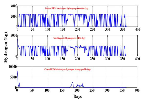
Figure 9.20: Central hydrogen production, hydrogen imported at HRSs and central storage profile (2,383 kg/day PEM central electrolyser (Cen. PEME Sc. 5)) under 2030-Cost scenario
