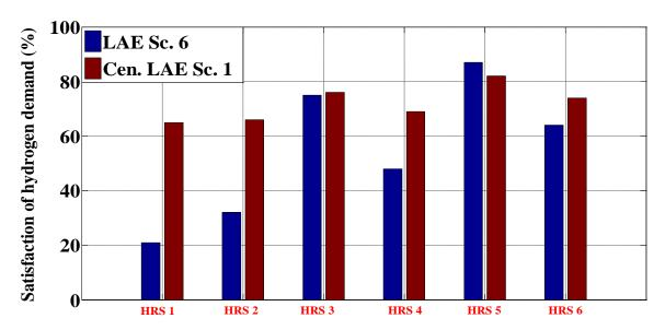
Figure 10.11: Comparison of Combination of HRSs and 1098 kg/day alkaline central electrolysers (LAE Sc. 6) and 2383 kg/day alkaline central electrolyser without electrolyser at the HRSs (Cen. LAE Sc. 1)
