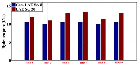
Figure 10.25: Comparison of Triple-sized default electrolyser size (LAE Sc. 20) and 6410 kg/day alkaline central electrolyser without electrolyser at the HRSs (Cen. LAE Sc. 8)
