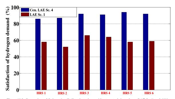
Figure 10.2: Comparison of Only onsite alkaline electrolyser without central electrolyser (LAE Sc. 1) and 6410 kg/day alkaline central electrolyser without electrolyser at the HRSs (Cen. LAE Sc. 4)
