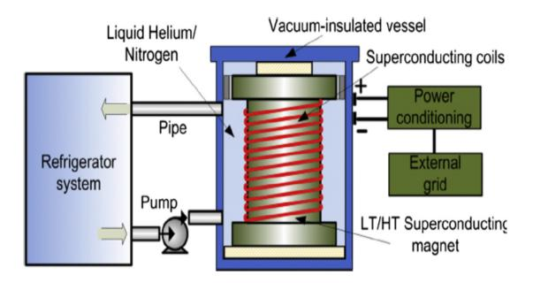
Figure 2.8: Superconducting magnetic energy storage
