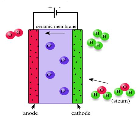
Figure 4.6: Principle operation of solid oxide electrolyte electrolysers (SOE)(Godula-Jopek, 2015)
