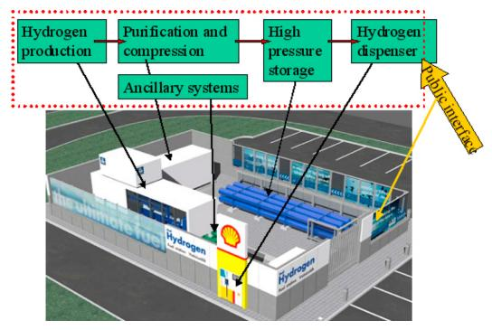
Figure 7.1: Hydrogen filling station parts
