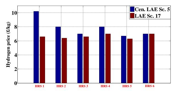
Figure 10.24: Comparison of Double-sized default electrolyser size (LAE Sc. 17) and 2383 kg/day alkaline central electrolyser without electrolyser at the HRSs (Cen. LAE Sc. 5)
