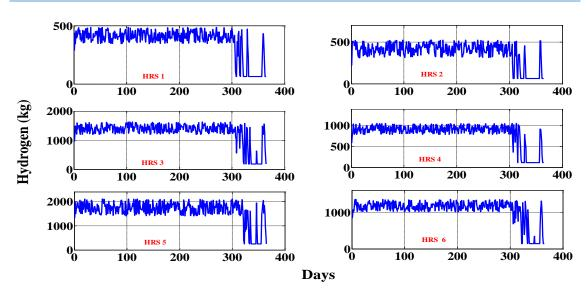
Figure 9.28: Daily variation of hydrogen level in storage tank throughout the year (5495 kg/day PEM central electrolyser (Cen. PEME Sc. 7)) under 2030-Cost scenario
