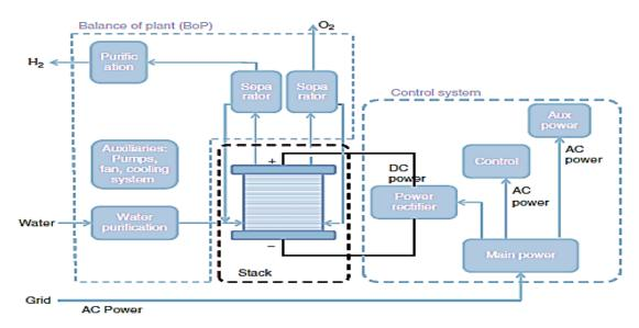
Figure 4.1: Water electrolysis diagram(Gandia, Arzamend and Diegnez, 2013)
