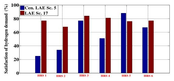
Figure 10.21: Comparison of Double-sized default electrolyser size (LAE Sc. 17) and 2383 kg/day alkaline central electrolyser without electrolyser at the HRSs (Cen. LAE Sc. 5)
