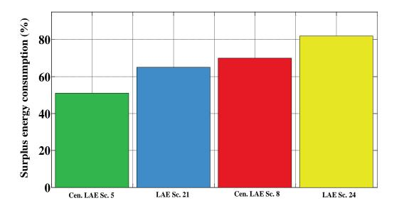
Figure 10.28: Energy consumption of Combination of HRSs and 1,098 kg/day (LAE Sc. 21), 4,853 kg/day (LAE Sc. 24) alkaline central electrolysers, 2383 kg/day (Cen. LAE Sc. 5) and 6,410 kg/day (Cen. LAE Sc. 8) alkaline central electrolysers without electrolyser at the HRSs energy consumption
