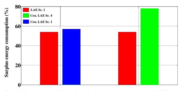
Figure 10.3: Energy consumption of Only onsite alkaline electrolyser without central electrolyser (LAE Sc. 1) , 2,383 kg/day(Cen. LAE Sc. 1) and ,6410 kg/day (Cen. LAE Sc. 4) alkaline central electrolysers without electrolyser at the HRSs
