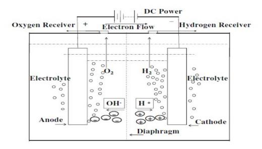
Figure 3.4: Water Electrolysis device
