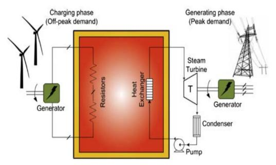
Figure 2.4: TES system integrated with wind power generation
