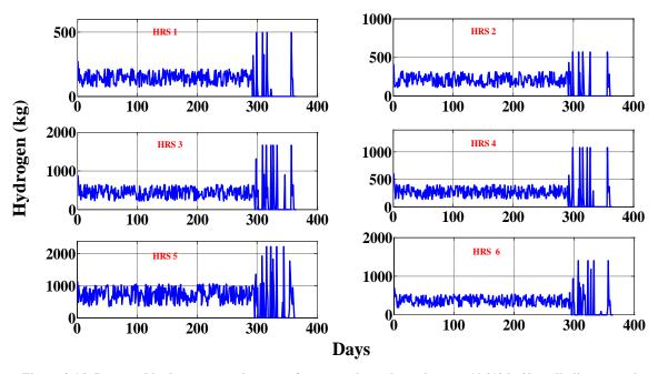
Figure 9.14: Imported hydrogen at each garage forecourt throughout the year (6,410 kg/day alkaline central electrolyser under 2015-Cost scenario (Cen. LAE Sc. 4))
