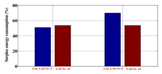
Figure 10.18: Energy consumption of Comparison of Only onsite alkaline electrolyser without central electrolyser (LAE Sc. 16), 2,383 kg/day(Cen. LAE Sc. 5) and 6,410 kg/day (Cen. LAE Sc. 8) alkaline central electrolysers without electrolyser at the HRSs
