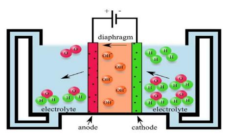
Figure 4.4: Principle operation of alkaline electrolyser(Godula-Jopek, 2015)
