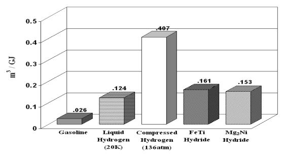
Figure 3.2: Volume of different fuels occupies for producing 1 GJ of energy
