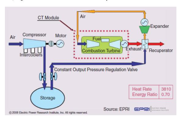
Figure 2.3: Main sections of a CAES plant
