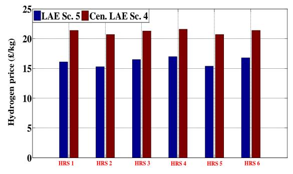
Figure 10.10: Comparison of Double-sized default electrolyser size (LAE Sc. 5) and 2383 kg/day alkaline central electrolyser without electrolyser at the HRSs (Cen. LAE Sc. 4)
