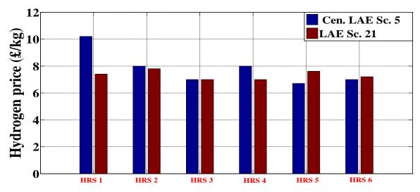
Figure 10.29: Comparison of Combination of HRSs and 1,098 kg/day alkaline central electrolysers (LAE Sc. 21) and 2,383 kg/day alkaline central electrolyser without electrolyser at the HRSs (Cen. LAE Sc. 5)
