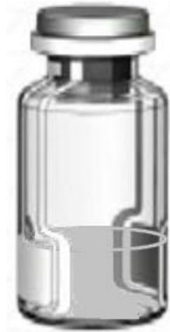
Figure 1 A schematic view of an impedance measurement vial with external electrodes containing sucrose 3% w/v.
