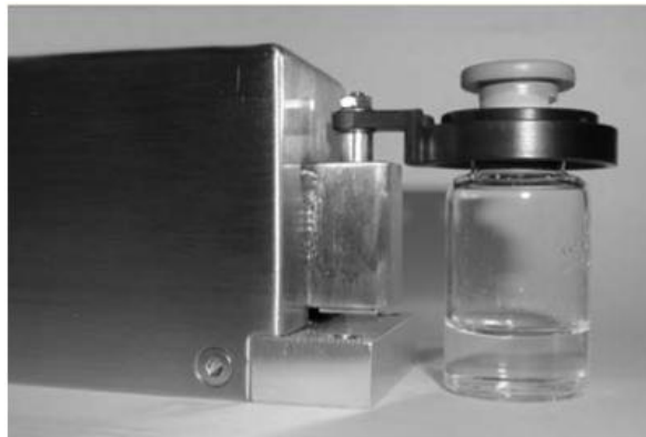
Figure 15 Microbalance with vial positioned in holding arm (Schneid, 2009)
