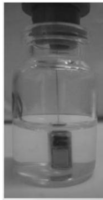
Figure 14 Vial containing temperature sensor for TempRIS (Schneid, 2009)
