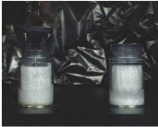
Figure 16 Photographic image showing sublimation front during primary drying of a sucrose solution (Chen et al., 2008)
