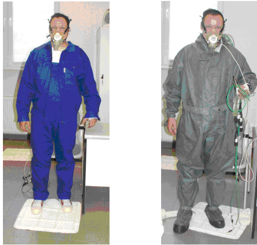
Figure 6.5. A cotton protective suit (left) or an impermeable coverall without head coverage (right) used in experiment of Marszalek (2006).
