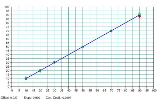
A3.2 Calibration curve for Paracetamol in Maize starch for the range 1524 – 1210cm<sup>-1</sup>
