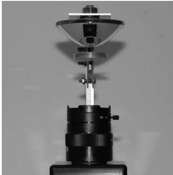
Figure 2.4: Single camera system video capturing equipment to generate stereo effect using a convex mirror and a concave lens (Yi and Ahuja, 2006)
