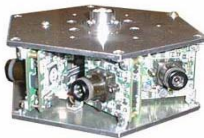
Figure 2.19: FlyCam (FX Palo Alto Laboratory 17 ): equipment to create Panoramic Video by stitching together images from multiple video cameras
