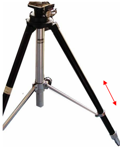
Figure 6.5: Adjustable legs of tripod suited to different-surface ground
