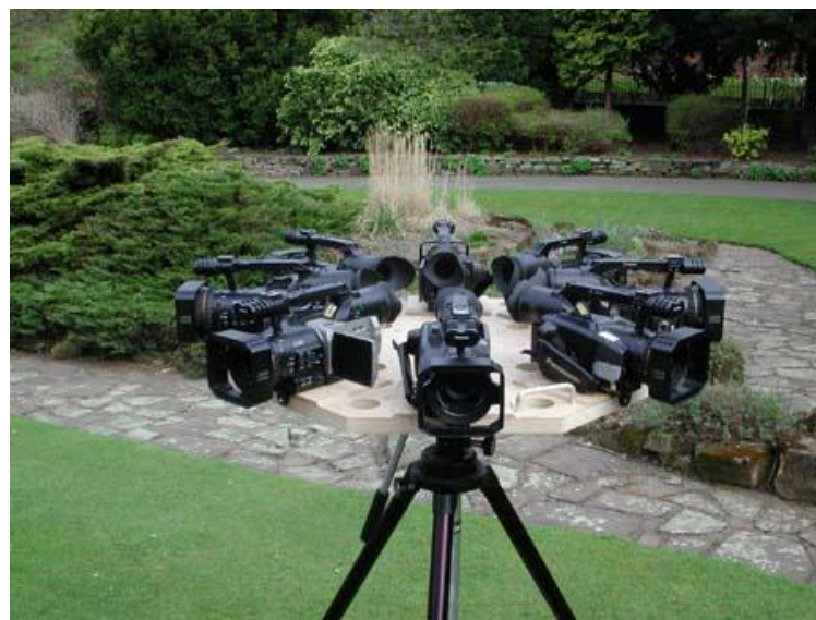
Figure 5, Eight Cameras to form a 360 degree view
