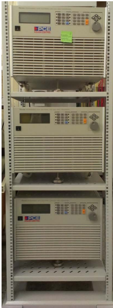
Figure 3-14: AC load bank consist of three Chroma 68306 programmable AC loads.
