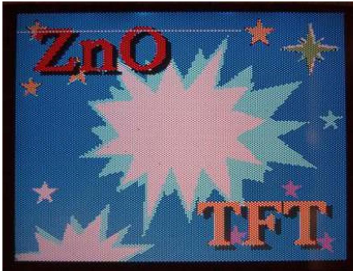
Figure 1.1 - A 1.46'' ZnO TFT driven LCD with improved picture and defect quality, demonstration from [8].
