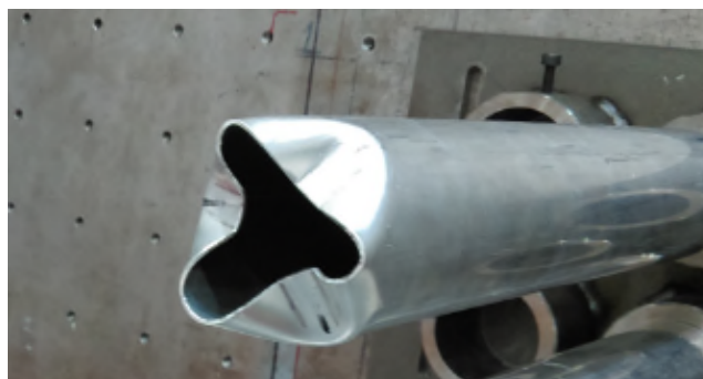
Figure 5 Tubes with three end notches as a trigger mechanism (Dimensions given in Table 1).
