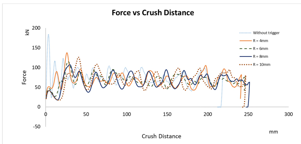
Figure 28 Force vs Crush Distance for circumferential notches with different radius.
