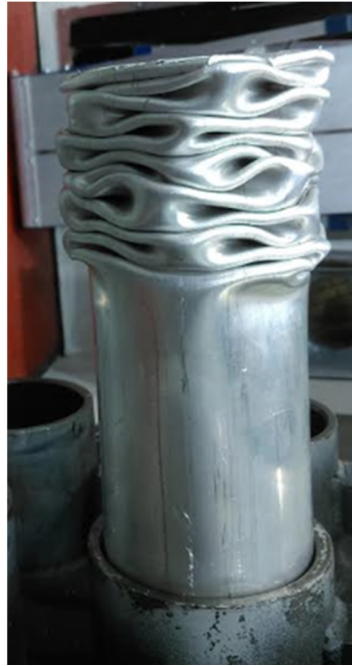
Figure 37 Deformed shape of the crash tube obtained in static and dynamic tests (Dimensions given in Table 1).
