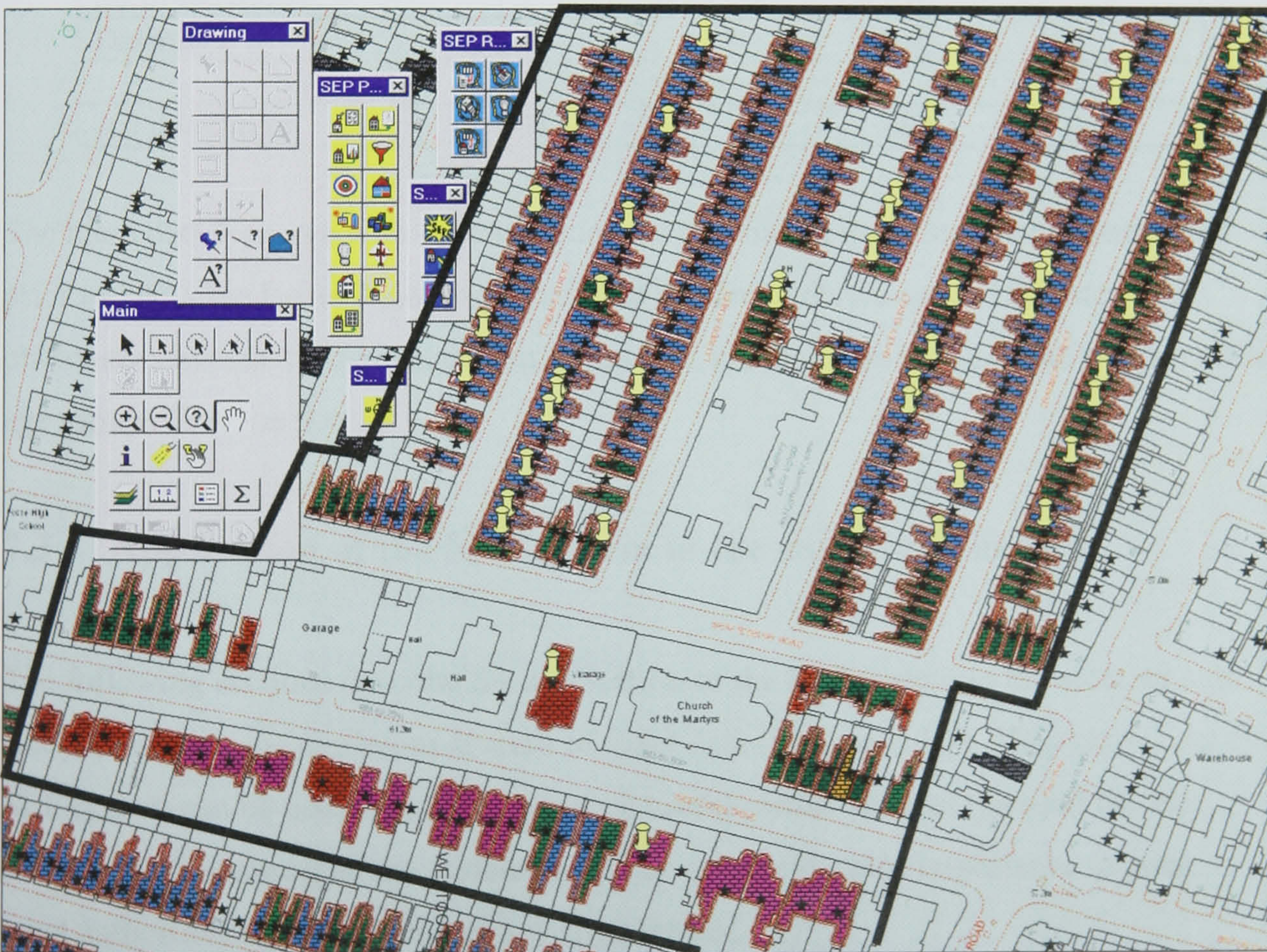
Figure 29. Case study area: the yellow pins indicate dwellings with Level 3 data. (N.B. where footprints are not coloured, the Footprint Tool was unable to automatically extract the dwelling footprint. These can be manually extracted by the system user.)
